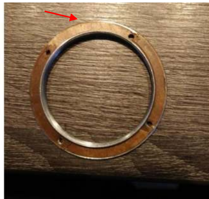
Attaching glue to keep the shims in place. The red arrow indicates the mark for the top of the lens mount.
