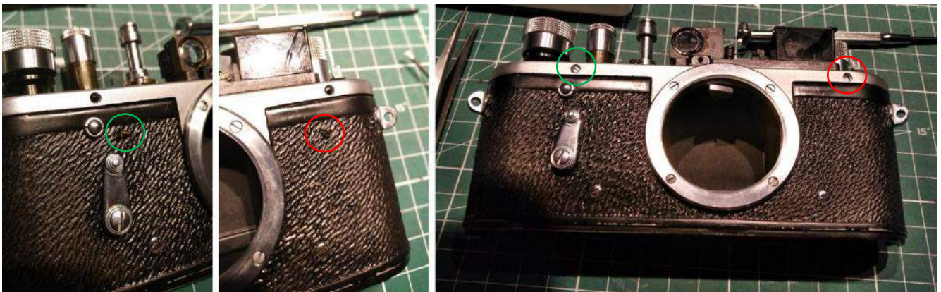
Securing the top plate to the body. Use the long screw (green circle) on the left and the short screw (red circle) on the right.
