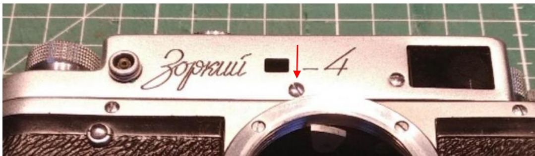
The screw indicated with the red arrow needs to be removed from the front.
