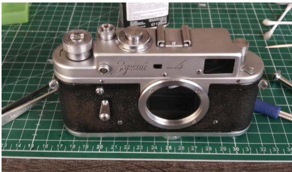
Securing the last screw. Note that the screw next to the viewfinder window is an access for the rangefinder calibration.
