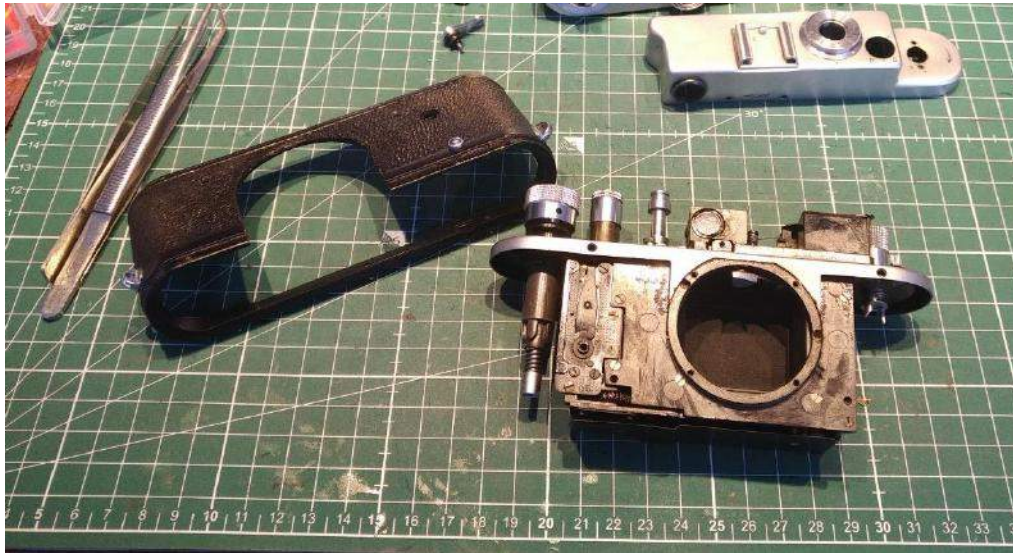
Shutter crate removed from the body.
