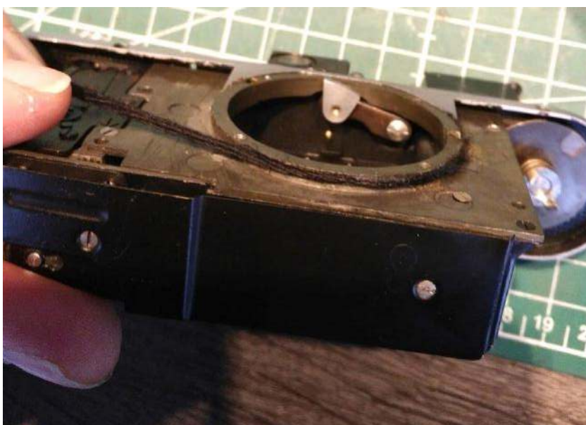
Getting the light seal into position.
