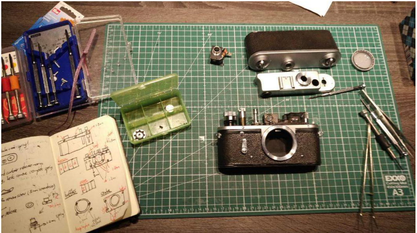
The state of reassembly just before the re-attachment of the slow-speed-mechanism. Note the sketches made during dismantling and the compartmented pill-box for temporary screw storage.
