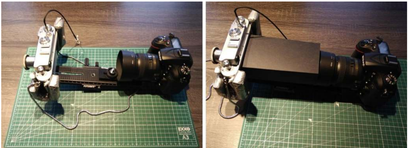
First step in creating the lightproof volume: adding a paper tunnel between the Zorki-4 focal plane and the take-up lens of the digital camera.
