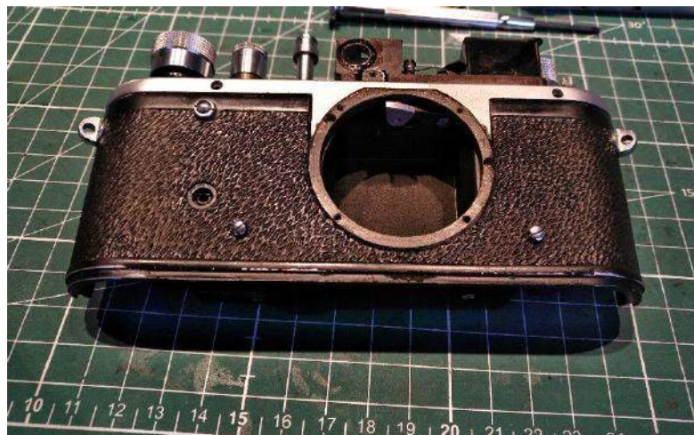
Shutter crate secured to the body.
