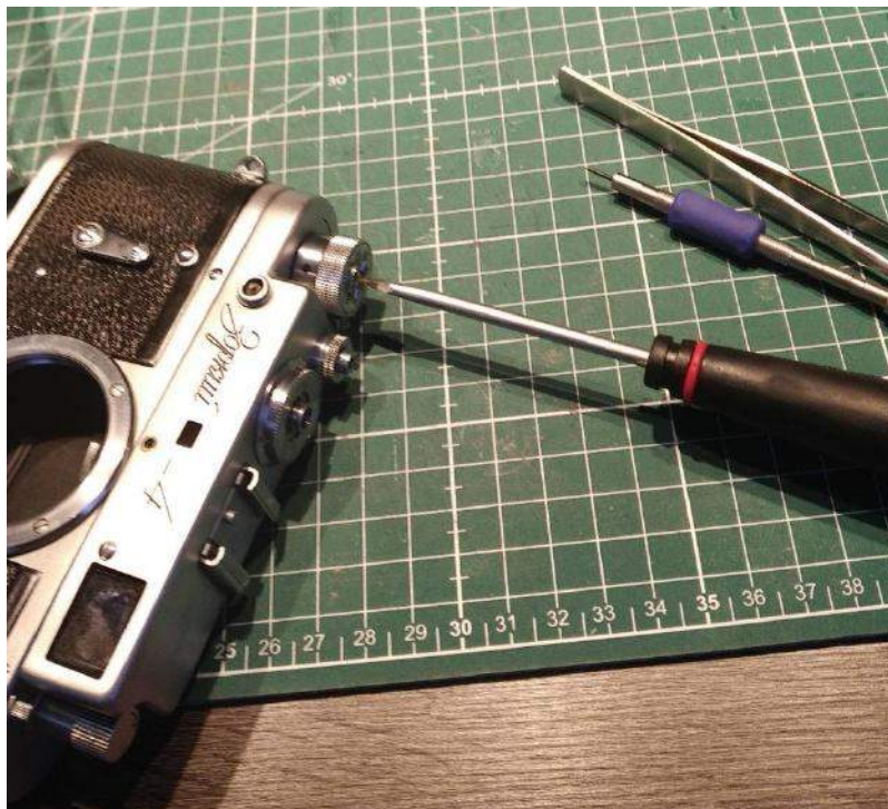
Removing the Zorki-4 winder knob top plate.
