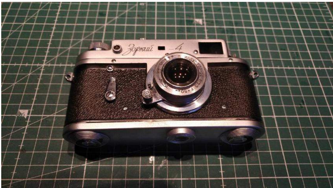
As a first step we'll unscrew the lens and store it in a safe place.
