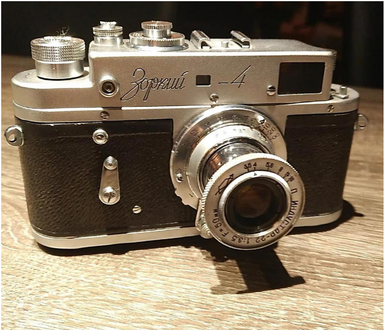
1961 Zorki-4 with Industar-22, retractable, 50mm f/3.5 lens.
