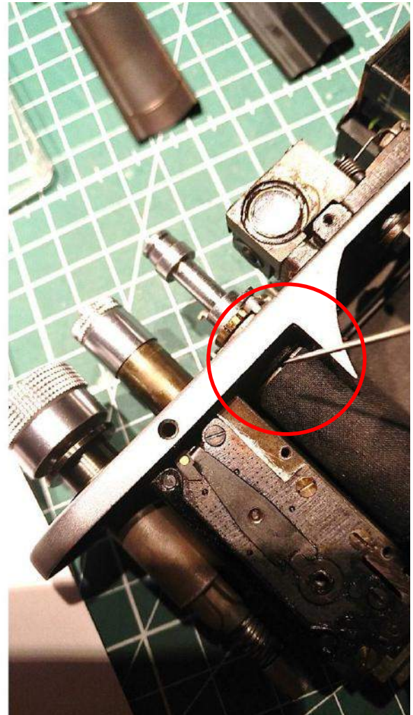
Lubrication of the shutter drum shaft. The red arrow in the left picture shows the tiny access for applying oil. The red circle in the right picture shows how oil is very carefully applied, using a needle.
