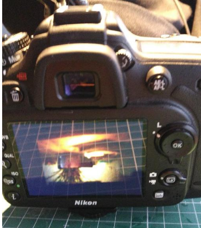
Image taken with the Zorki-4 and Nikon D7200 test setup (the image is upside down and left-right reversed of course).
