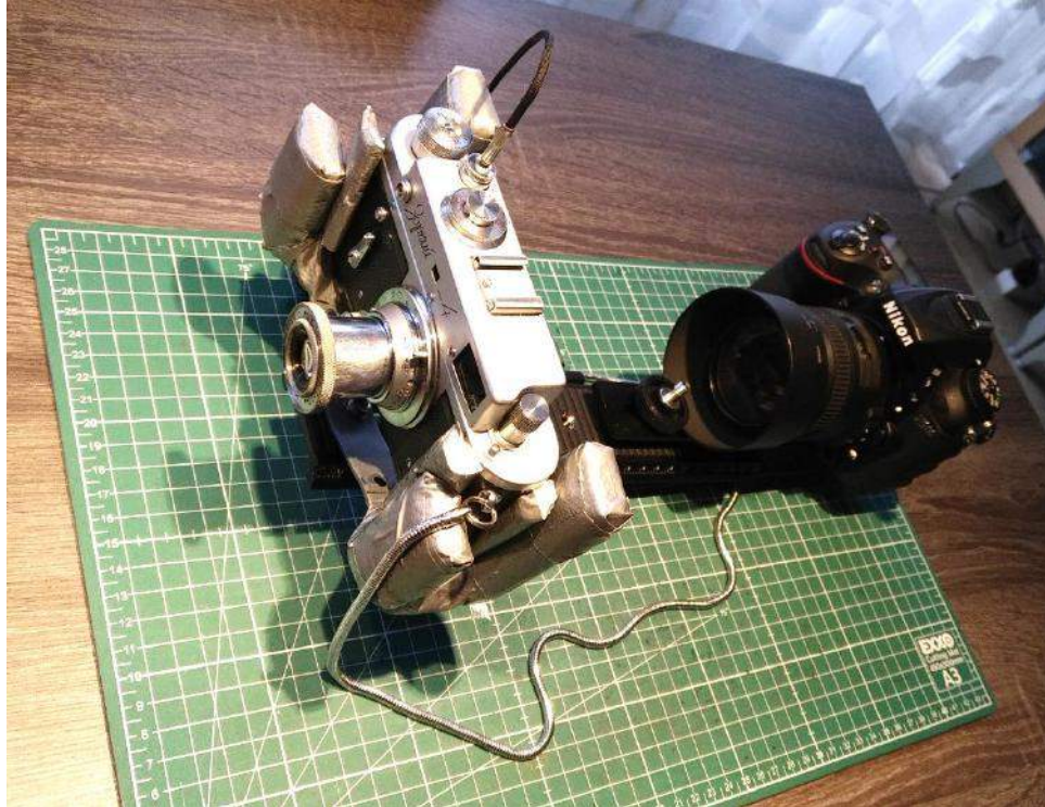
The rig shown from another angle. Note the small cushions made to position and tighten the Zorki-4.
