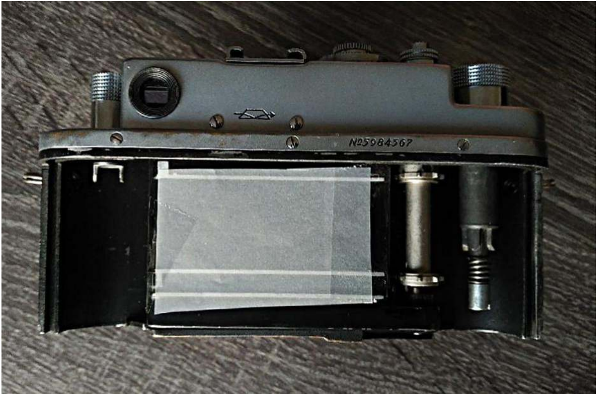
Tracing paper is attached to the 'film-plane'.
