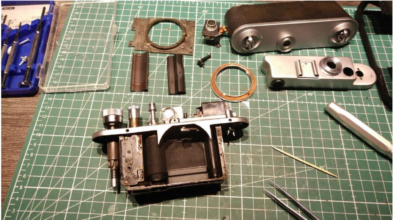
Opened-up shutter crate with above the two light baffles and above that the crate front.
