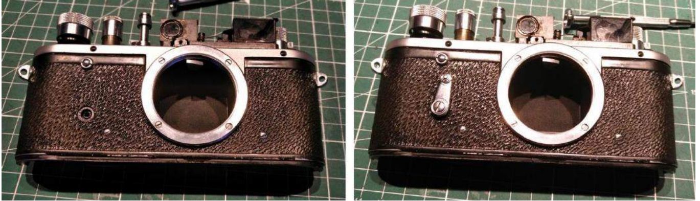
Reattaching the self-timer lever.
