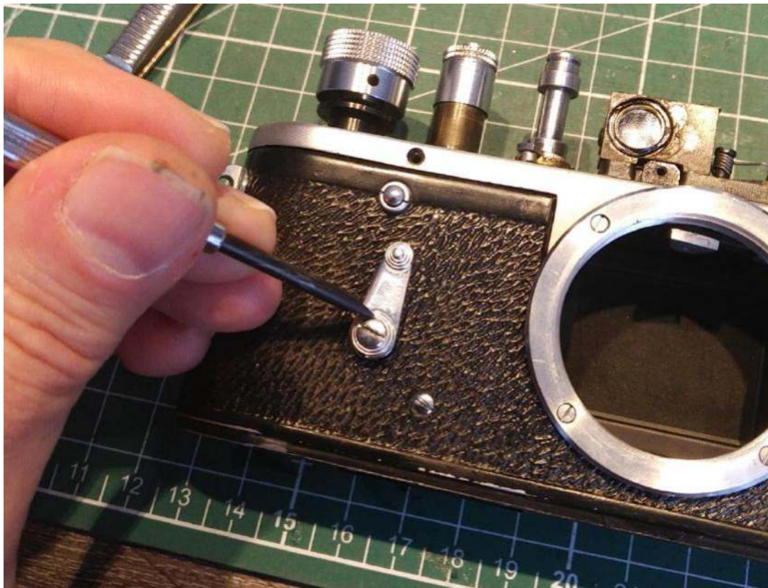
Removing the self-timer lever.
