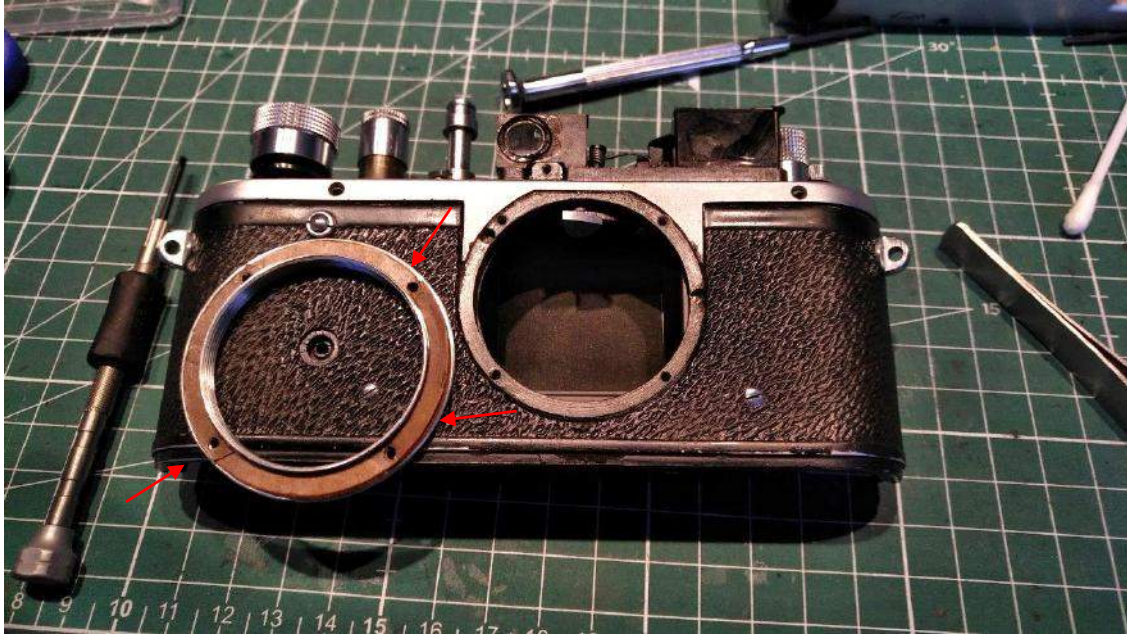
The loose shims (red arrows) need some attention.
