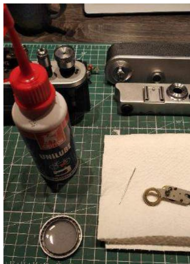
Lubricating, using sewing machine oil and a needle. The lid of a 35mm film container forms a handy oil reservoir.
