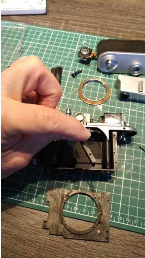
Replacing the light baffles. Don't worry too much about the exact placement.
