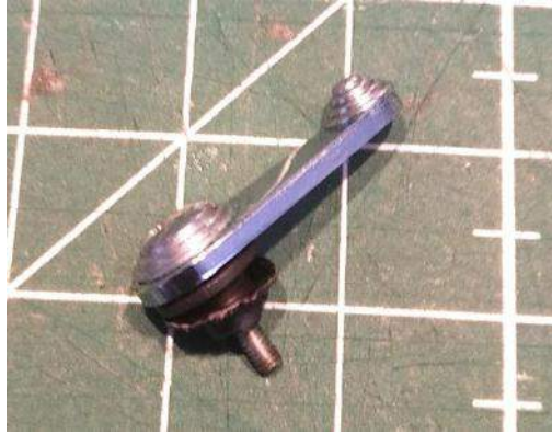
Self-timer lever with light seal taken out.
