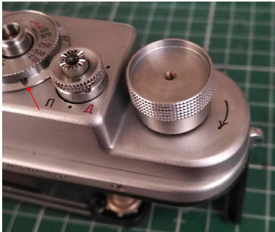
Securing the rewind knob by turning it clockwise and securing the shutter speed indication ring (see red arrow).
