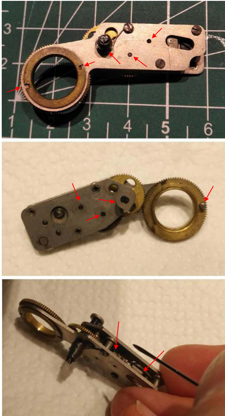
Lubrication points for the slow-speed-mechanism (red arrows).
