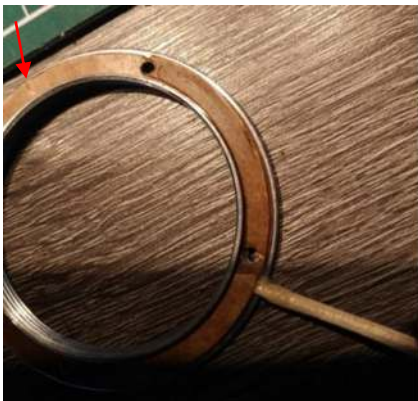
Attaching glue to keep the shims in place. The red arrow indicates the mark for the top of the lens mount.
