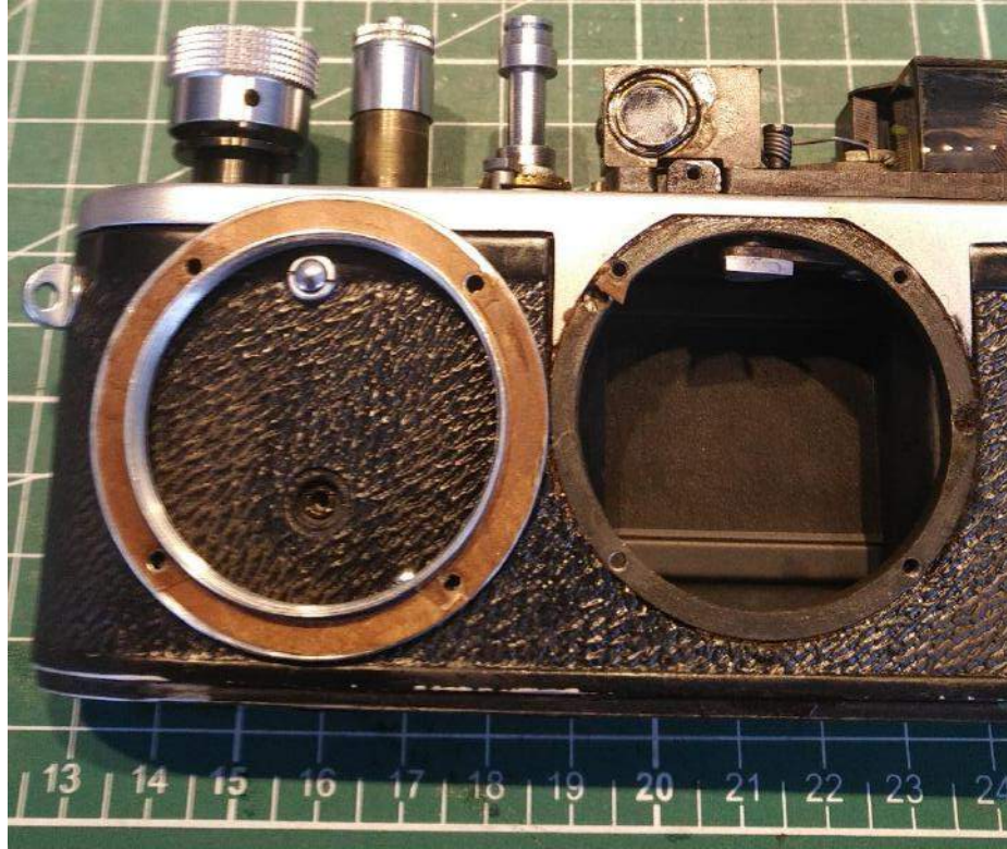
Shims underneath the lens mouth.
