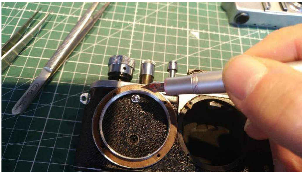
Marking the shims positions and the top of the lens mount itself.
