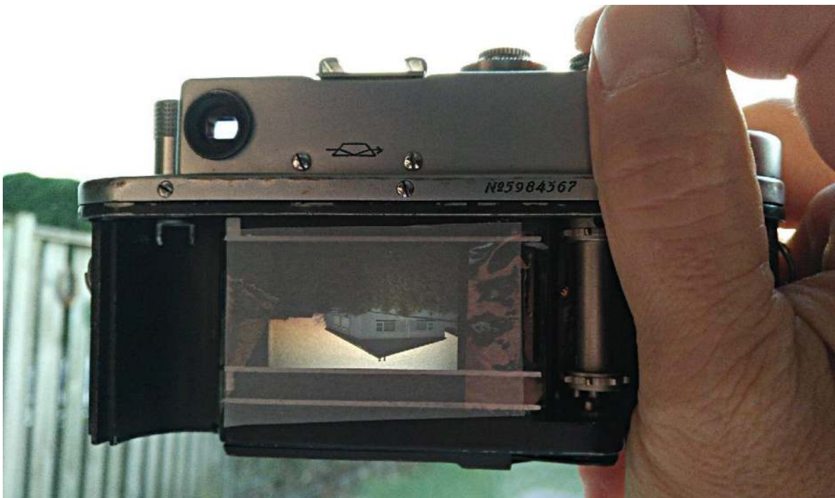
With the aperture wide open, the shutter speed on B and the shutter pressed, the image is visible on the tracing paper and can be checked for focus.
