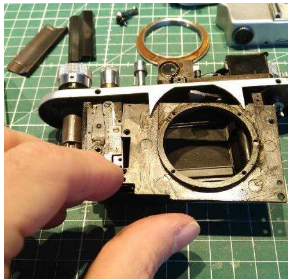
Replacement of the shutter crate front.
