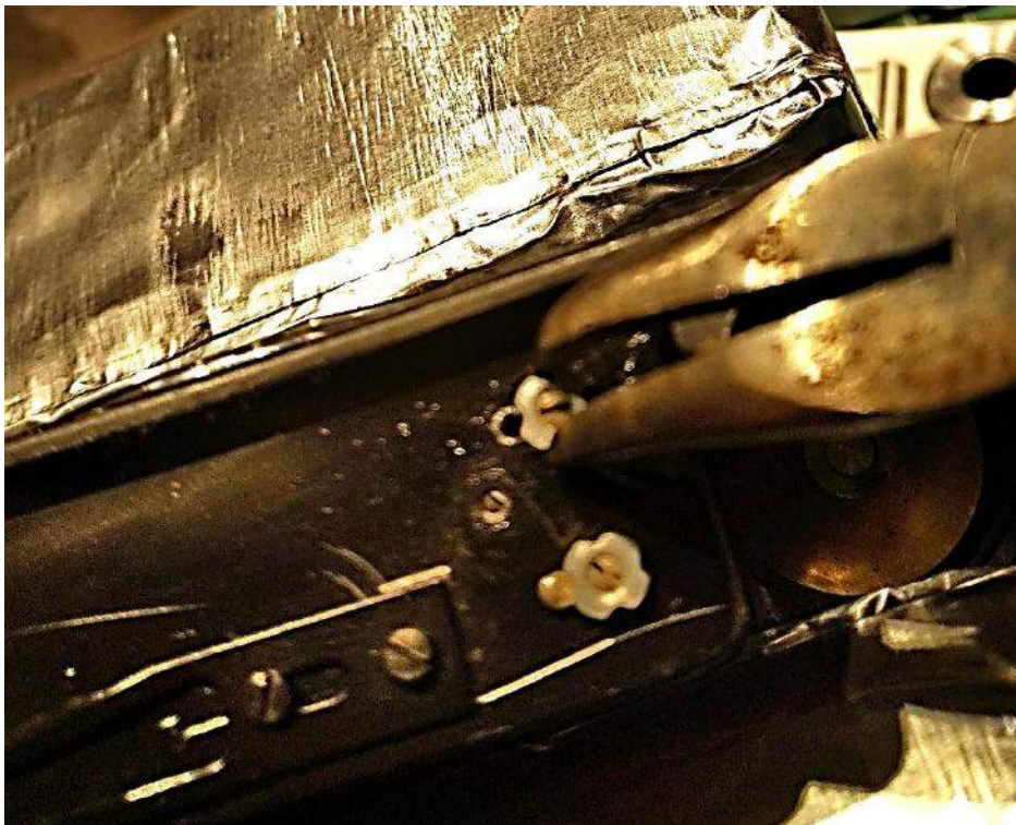
Adjusting the curtain tension. Shown here is an adjustment of the second curtain tension.
