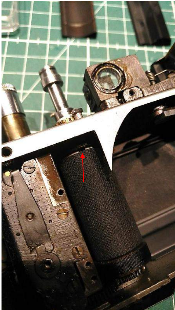
Lubrication of the shutter drum shaft. The red arrow in the left picture shows the tiny access for applying oil. The red circle in the right picture shows how oil is very carefully applied, using a needle.
