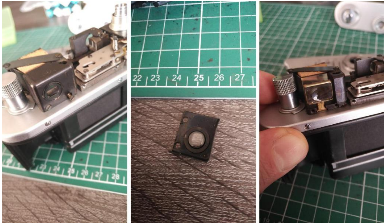
Removing the viewfinder window to get a better access to the viewfinder.
