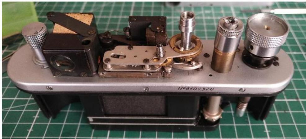
Secure the slow-speed-mechanism with two screws.
