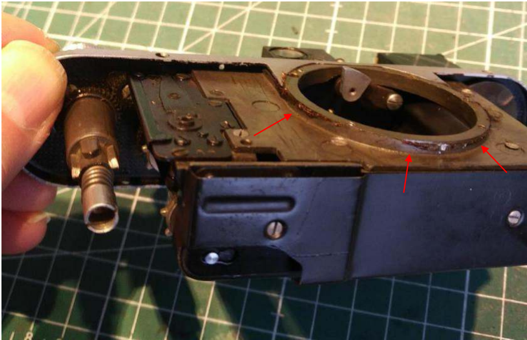
Remove the remnants of seal (thread) and glue.
