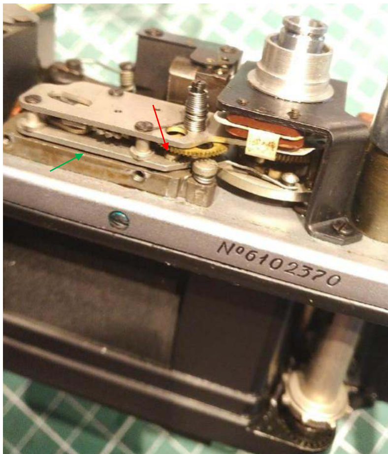
The slow-speed-mechanism underneath the flash-synchronization-switch. Note the screw underneath the large gear (red arrow) and the use of spacers (green arrow).
