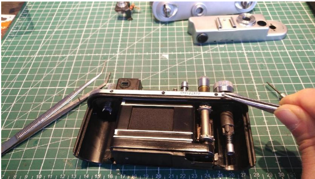
Removing the three top plate screws on the back of the Zorki-4.
