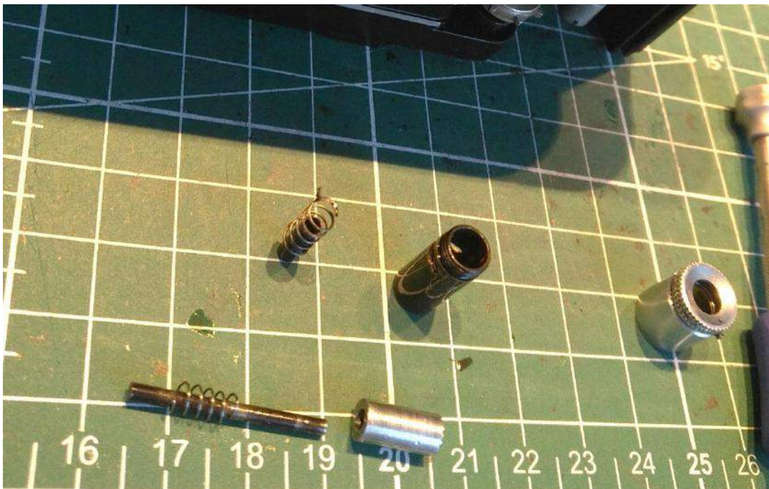
Disassembled shutter-rewind mechanism. Note that the screws are loosened, not removed.
