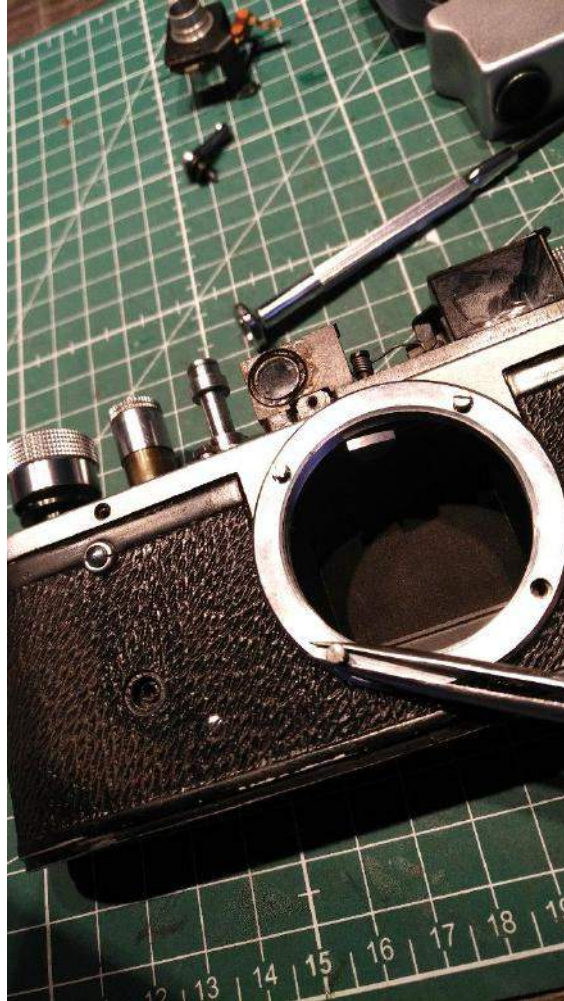
Using a pair of tweezers may aid in attaching the lens mount screws.
