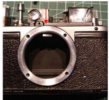
Attaching glue to keep the shims in place. The red arrow indicates the mark for the top of the lens mount.
