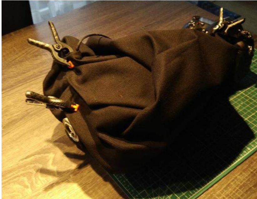
Setup wrapped in black cloth to make it lightproof.
