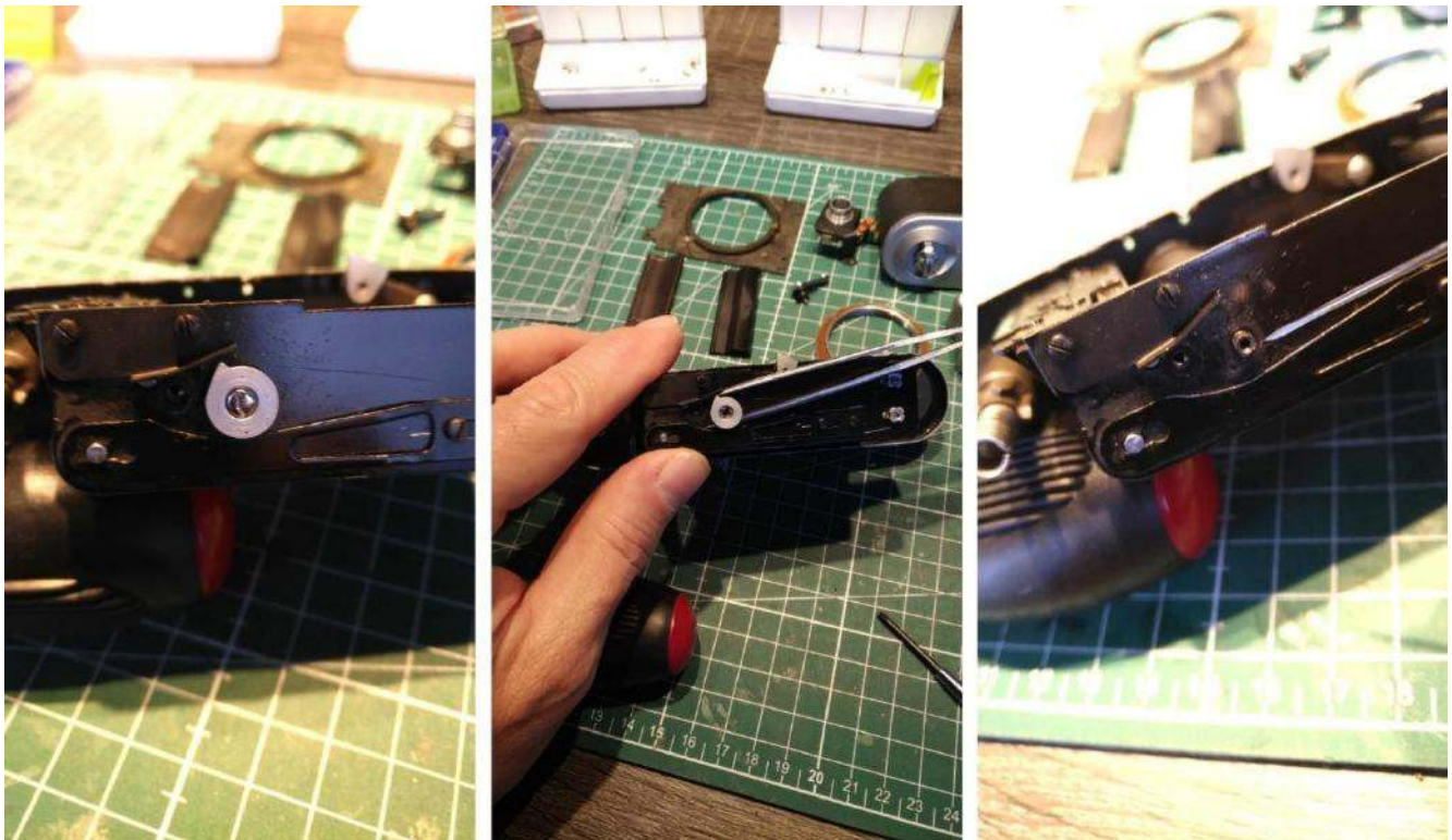
Shutter latch removal and oiling of the bottom drum shaft pivot.
