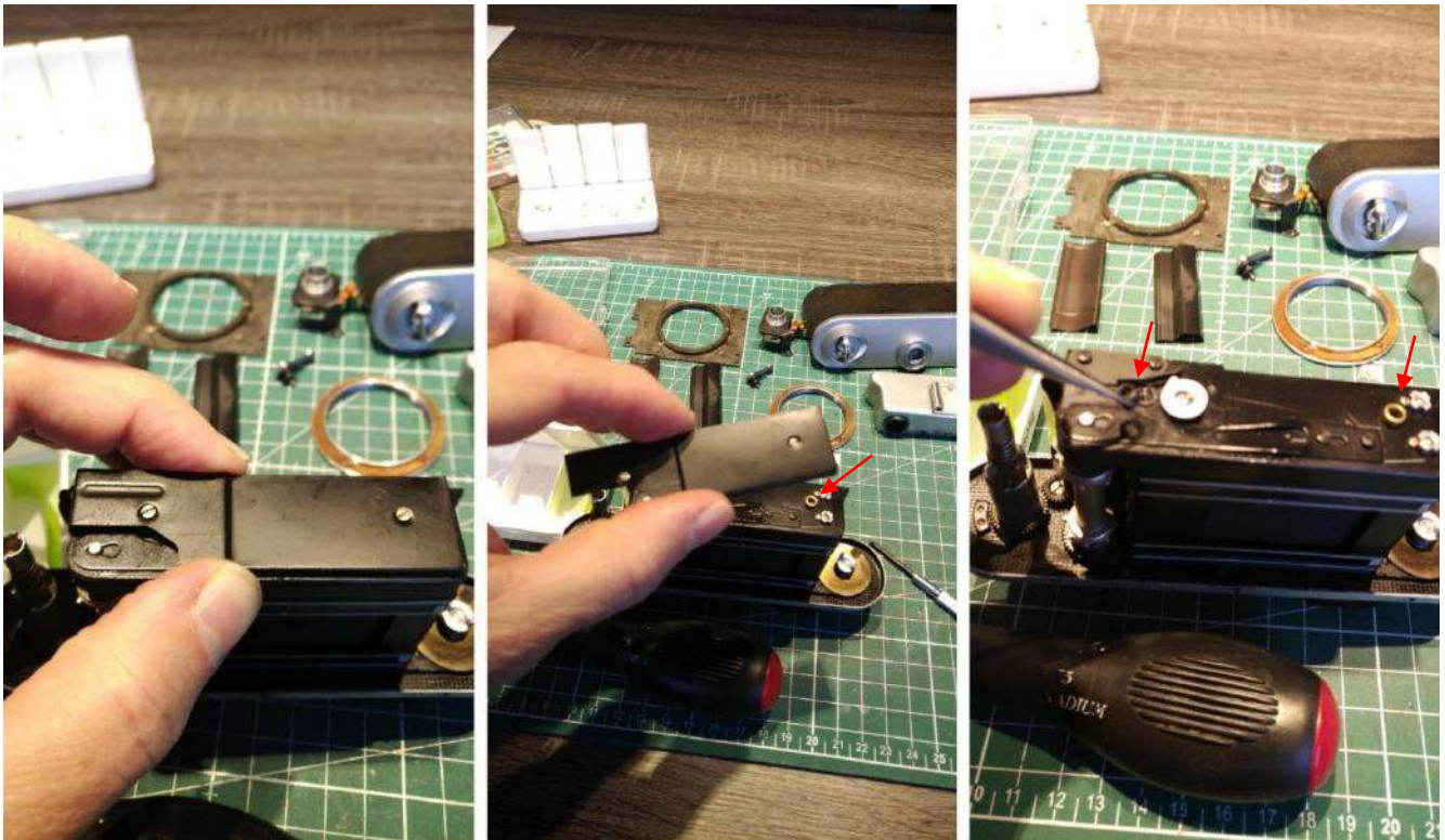
Removing the bottom cover. Notice the brass shim on the right and the black shim (in tweezers) on the left (red arrows).
