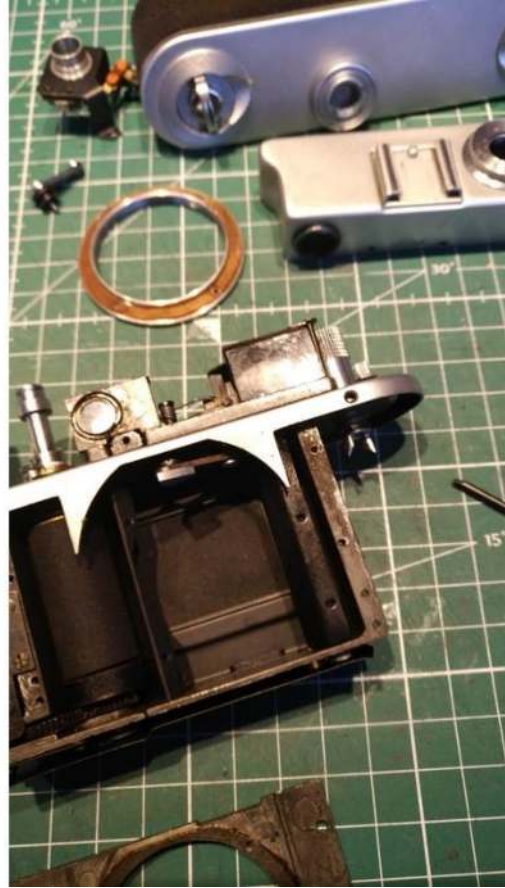
Replacing the light baffles. Don't worry too much about the exact placement.
