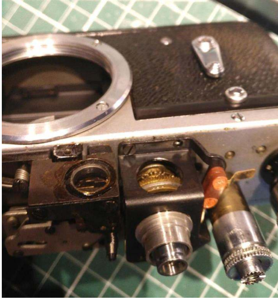
Front view showing the flash-synchronization-switch over the slow-speed-mechanism.
