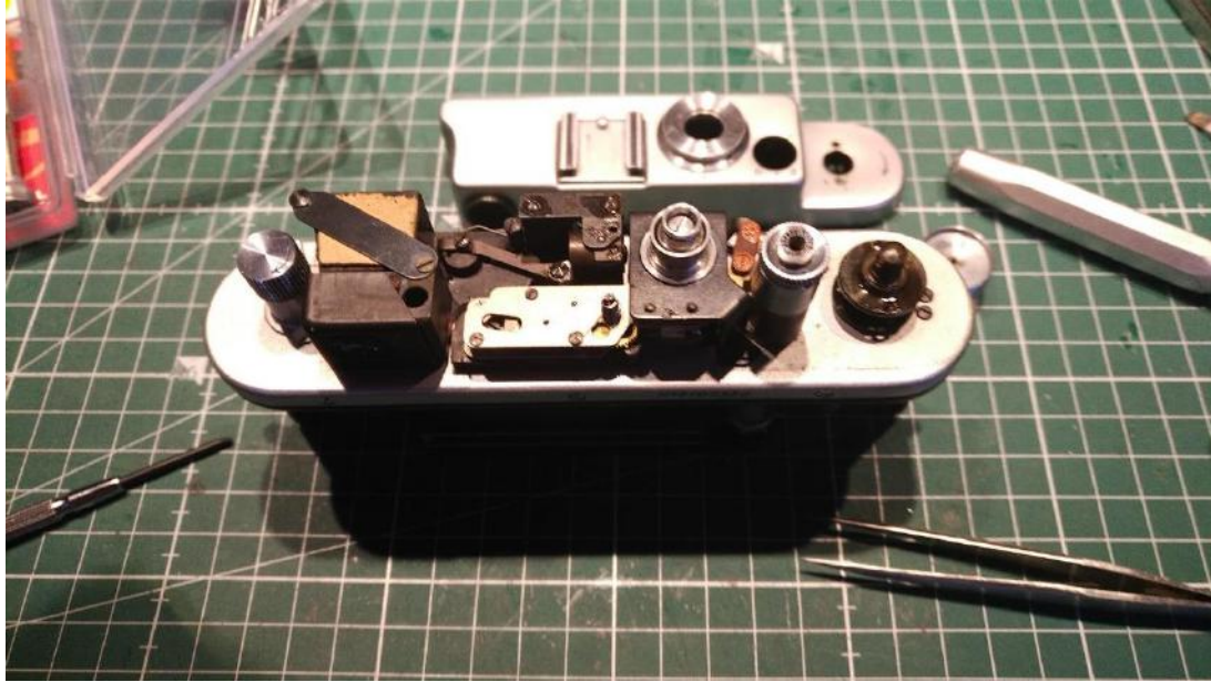
Zorki-4 with top removed. Note that the synchro ring is loosened but still in place.
