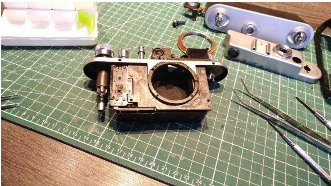
The light baffles secured.
