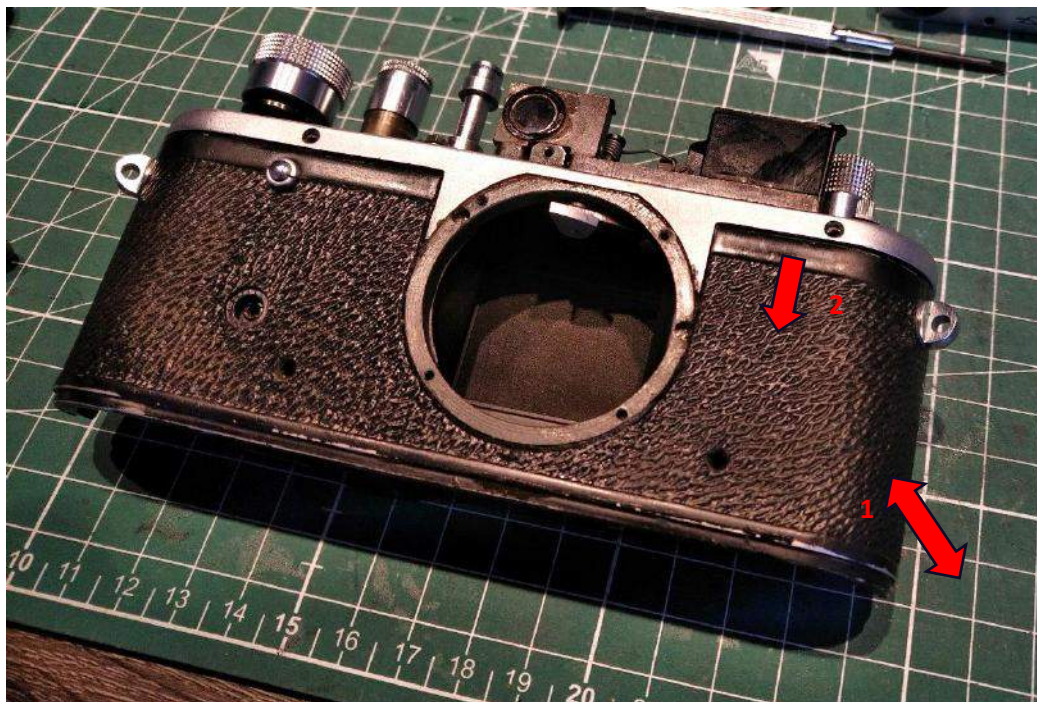
Wriggle the bottom of the body (1) to slip the top plate off (2).
