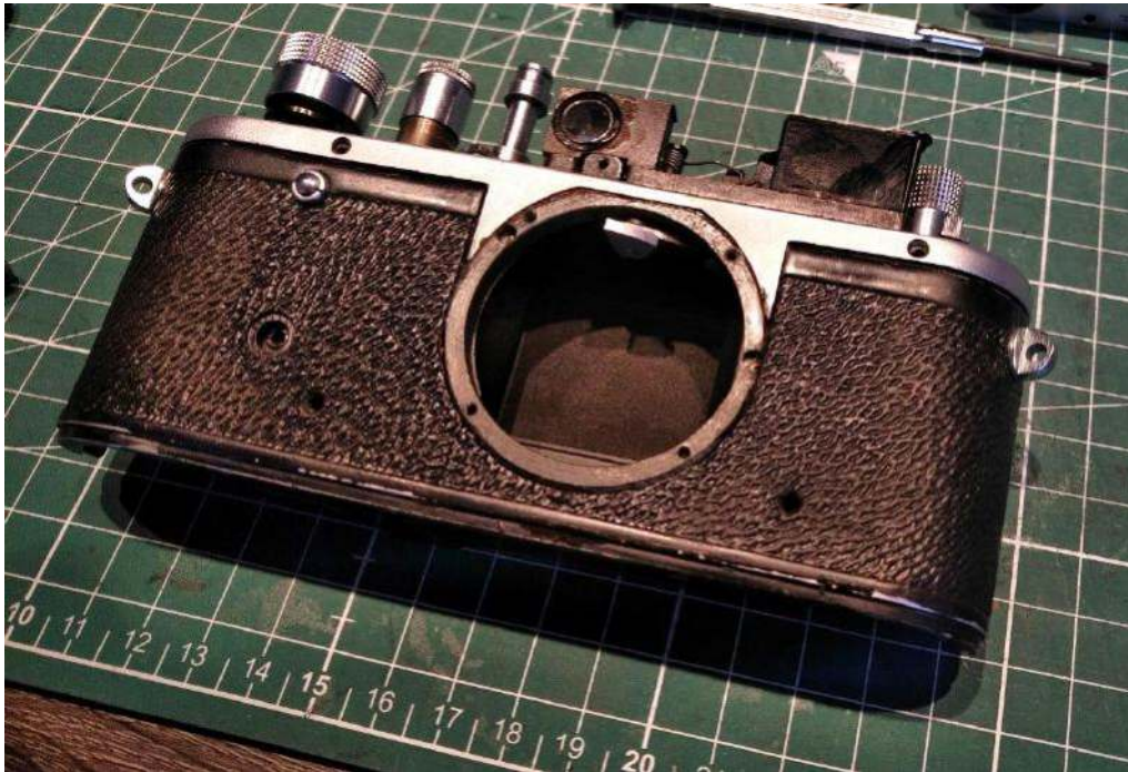
Shutter crate with new light seal pushed back into the body.
