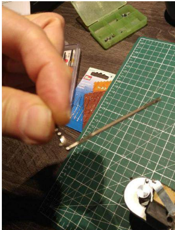
Clean and lubricate the second curtain release arm with thin oil before replacing it.
