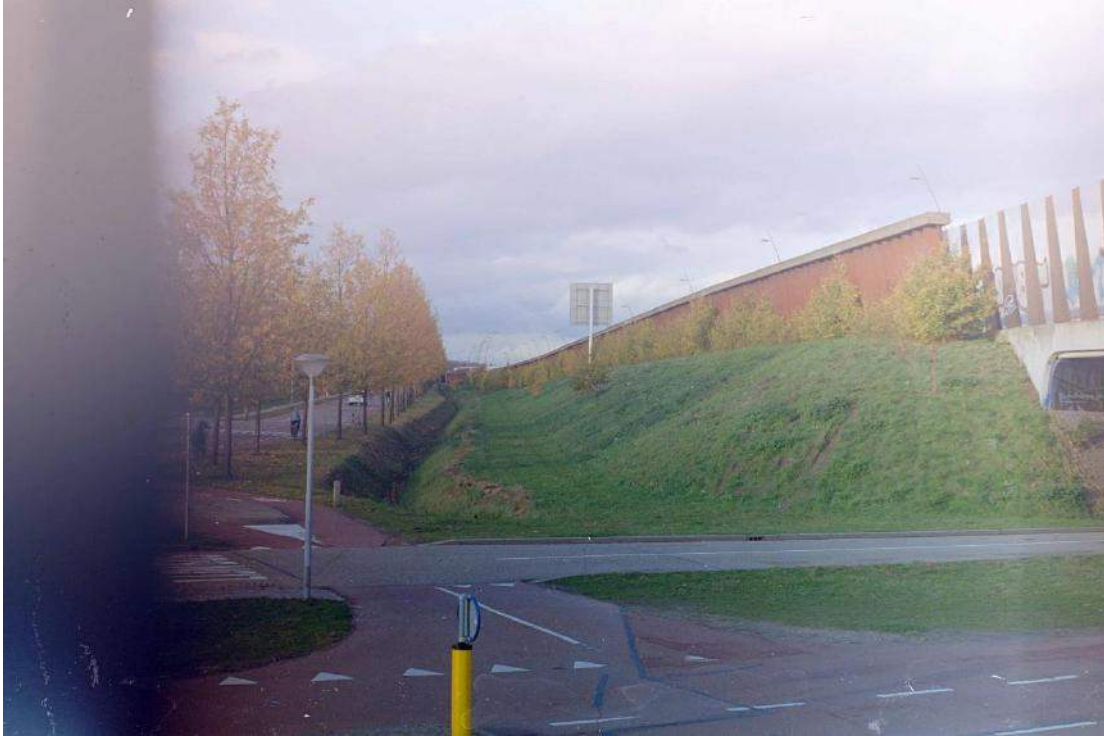
Effect of lagging shutter curtains, noticeable in the uneven exposure on the left and – to a lesser extent – on the right of the frame. Picture taken with a FED-3 camera, having a shutter nearly identical to the one of the Zorki-4.
