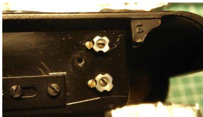
Second curtain (top) and first curtain (bottom) tension adjustments screws.
