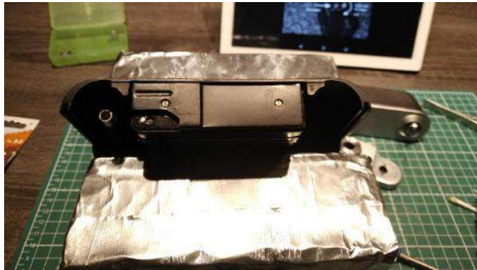
Camera in upside-down position in a makeshift hold. The bottom cover of the shutter crate needs to be removed. Use a 2.4mm screwdriver and note the positions of the shims.
