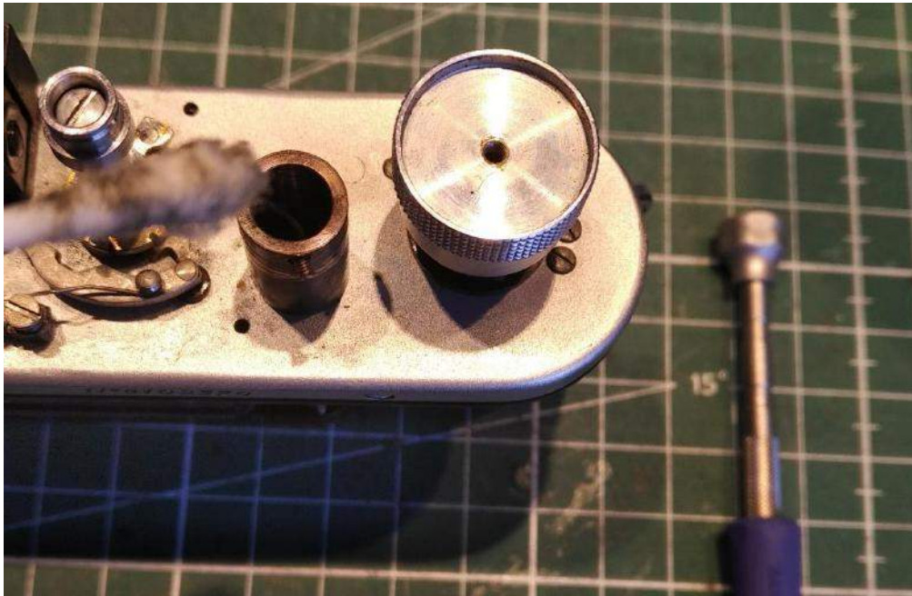
Cleaning the shutter-rewind mechanism shaft.
