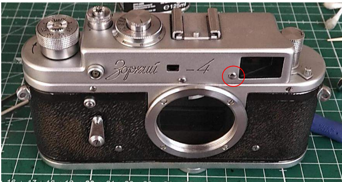
Remove the screw in the red circle to get access to the rangefinder calibration screw.
