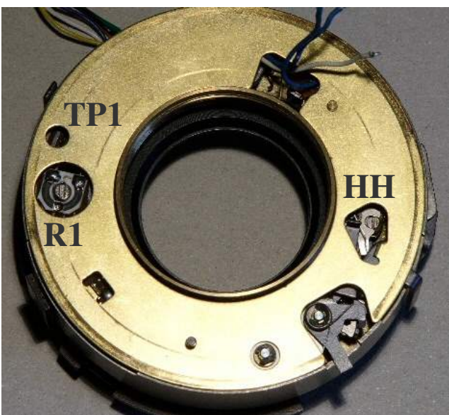
PIC 40: Front cover ring: note the holes to access the trimmer R1 and test point TP1 (see PIC 37). Note also the access to the screw to adjust the device HH (see PIC 28 and 31).
