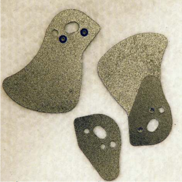
PIC 14: Normal blade (upper left), reversed blade (upper right), special blade (bottom)
