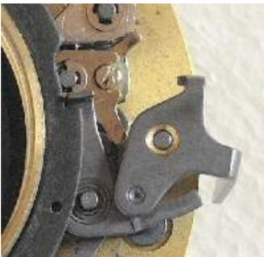
PIC 19: Hook lever T engages cogged ring R .
