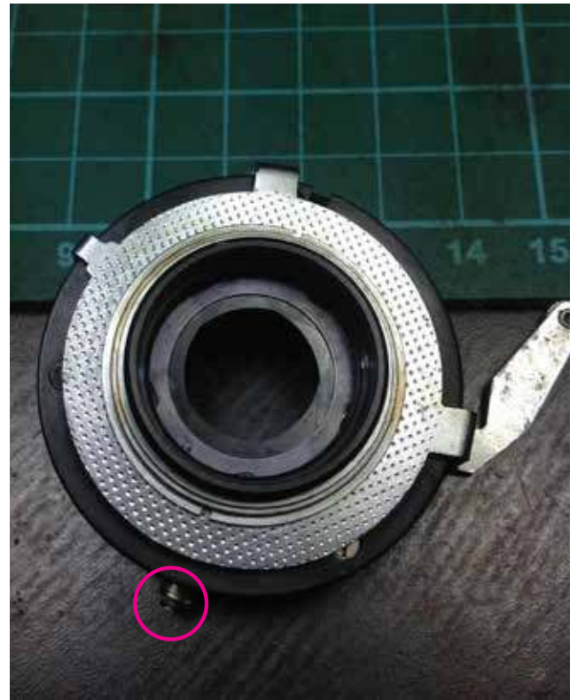
10: The sync cable post on the shutter side HL in red. Note the back side position of the cocking lever and aperture selector. You'll remove it later if you decide to dig deep.
