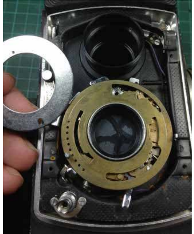
02: Once the cover plate is removed, study the speed plate position. At this stage you can test how it moves while holding it down.
