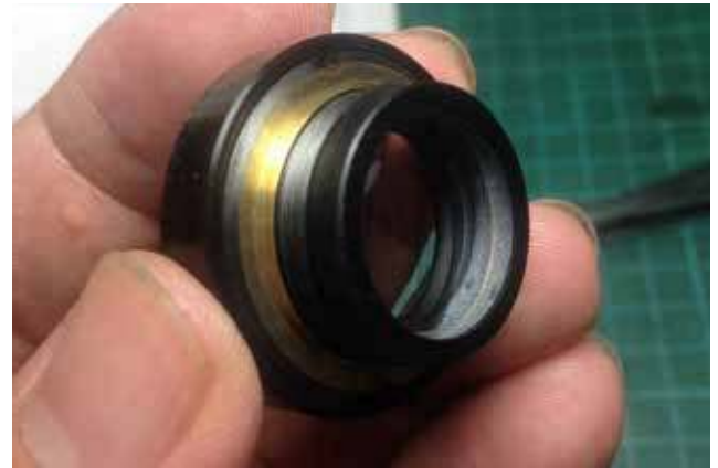
02: inspect the front lens elements front and back side. I make it a point to immediately clean it with glass cleaner using cotton buds and then wiping it off with a clean lens tissue. The set aside.
