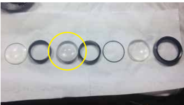
03: I removed the viewing lens elements and in turn they all come apart (pictured) be sure to remember where each once goes. It is very IMPORTANT. I made the mistake of putting back the middle lens (highlighted HL, in yellow) the WRONG way and the focus is off once assembled.
