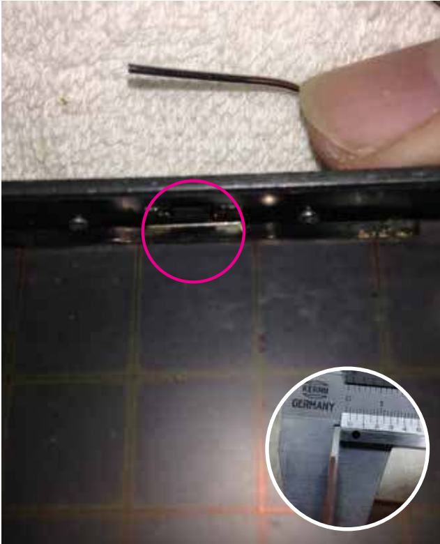
07: Push down this metal clip and slide outward to remove. Be gentle as the glass is thin (around 1.2mm see insert). Take note of rusted metal parts. In this case you need to scrape and touch up with black & silver paint accordingly. Take out the mirror.
