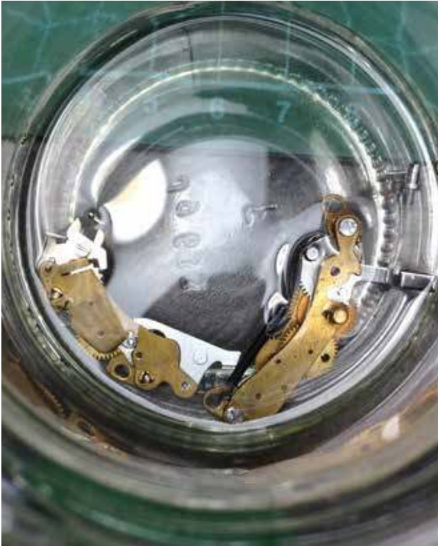
13: I put both the ST and SSE mechanism in a lighter fluid or ronsonol bath. I use a bristle brush to wipe it while submerged. You can do this several times while taking it out for a test run on all their gears. I did it thrice each time with a fresh fluid batch.
