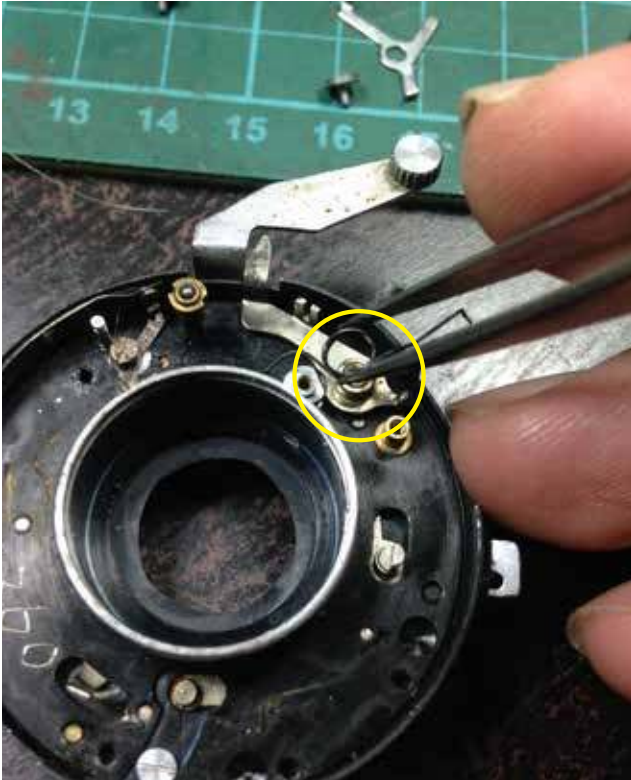
19: Once again note the spring HL in yellow of the shutter release lever. Take note of its position in relation to the shutter housing.
