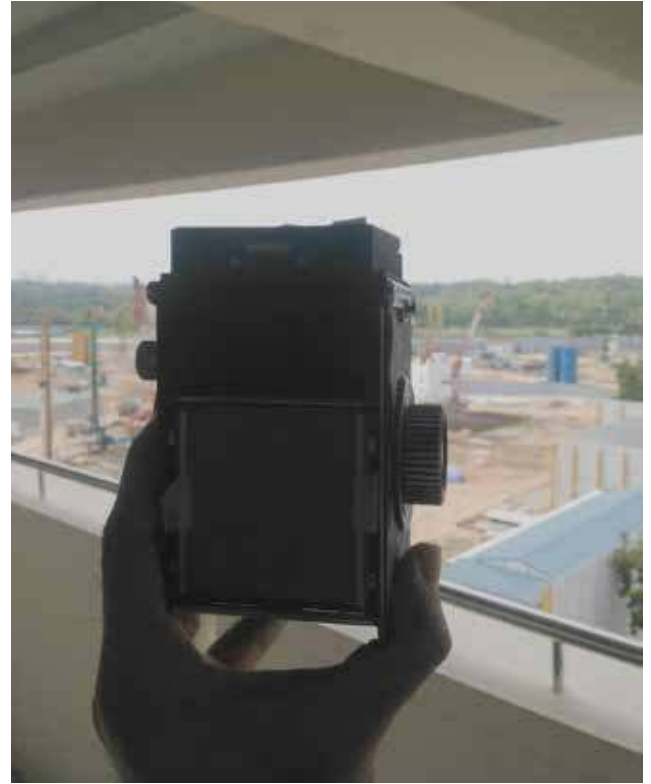
15: Since without the back plate there is no more tripod mount, I just handheld and with a bit of dexterity try to view from a distance and see if the view is sharp. This part is trial & error and might take you several tries before getting the focus right. See and do step #8 after each viewing.
