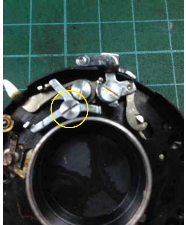
14: Now pardon my terminology on these section. Start with this lever. Do note that this is in sequence for easy removal. Loosen the big screw HL in yellow and take note of the spring below. Mark its position.
