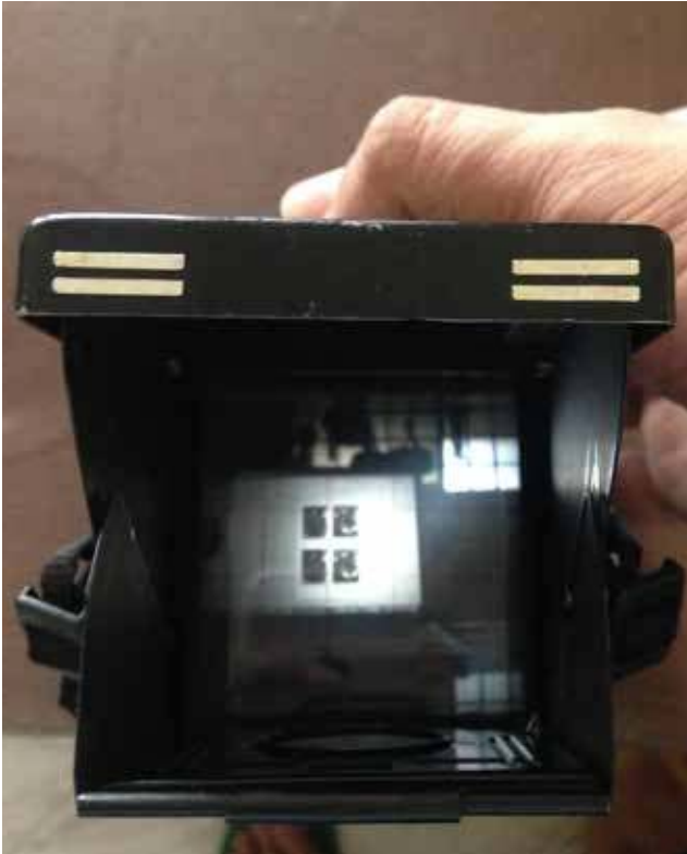
18: Now open the viewfinder and hold the lens with your right hand try to adjust the lens position. Do this slowly in small increments, once you hit the focus sharp on viewfinder you're almost done.
