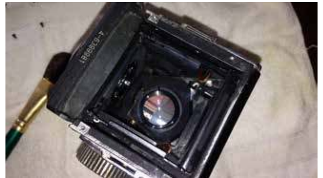
02: Here you can see the angled mirror that allows you to see through the taking lens. Inspect the internal parts for obvious dust and dirt. Watch out for rusted metal parts as well.
