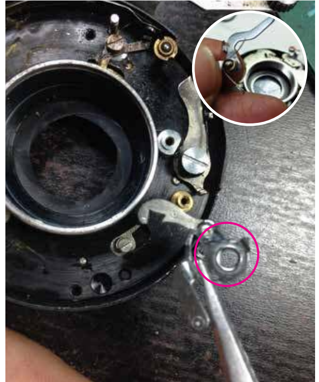
16: As you can see there is no spring underneath HL in red. See inset photo of a Prontor lever with spring as reference. Maybe the previous owner or repairman tried and failed in putting this back together. Reason why many missing parts. Now this is where the second donor unit comes into play. Without the donor unit this build is a bust. See NOTES section at last page.
