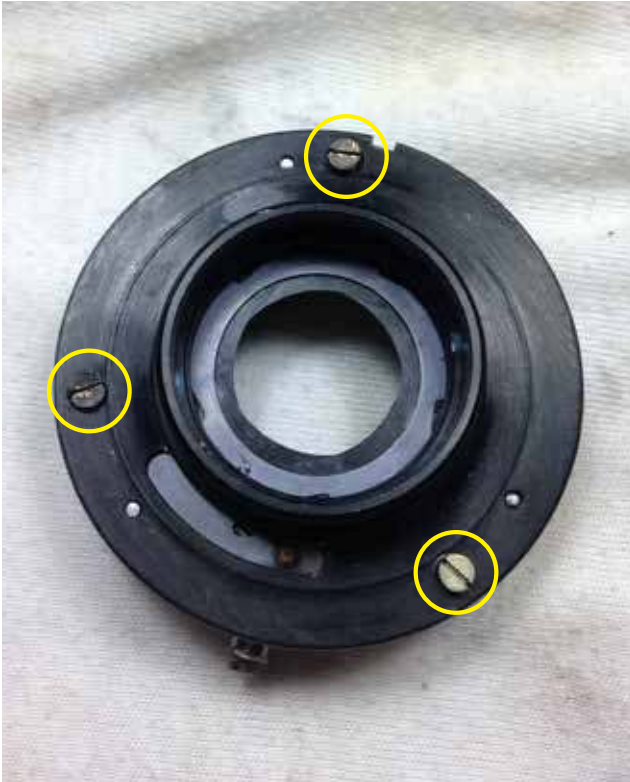
01: Back side of the shutter body has three screws HL in yellow. Remove them take note of the position which screws goes to which hole.
