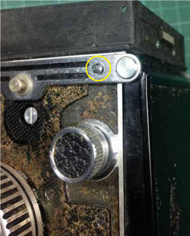
10: This section is to show how you go about doing ground glass focusing at the back of taking lens. Start by loosening the screw HL in yellow to remove the back cover plate.
