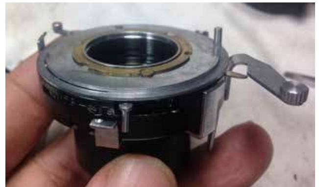
06: Inspect the ST escapement mechanism. Make sure it works. This one has some rust spots and needs light scraping. Do note where the spring was placed. You might need to de-rust this parts using whatever available means you can. I have a dremel so it helps.
