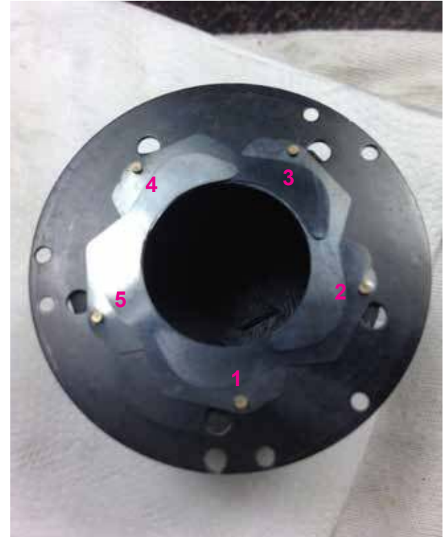
12: So study procedure #10 again and take note of the HL parts. So here we are this time I numbered them accordingly. Start with #1 from the bottom and work your way counterclockwise.. Once you're at #4 pay attention on how to put it underneath #1. And the same with #5. See end result here.
