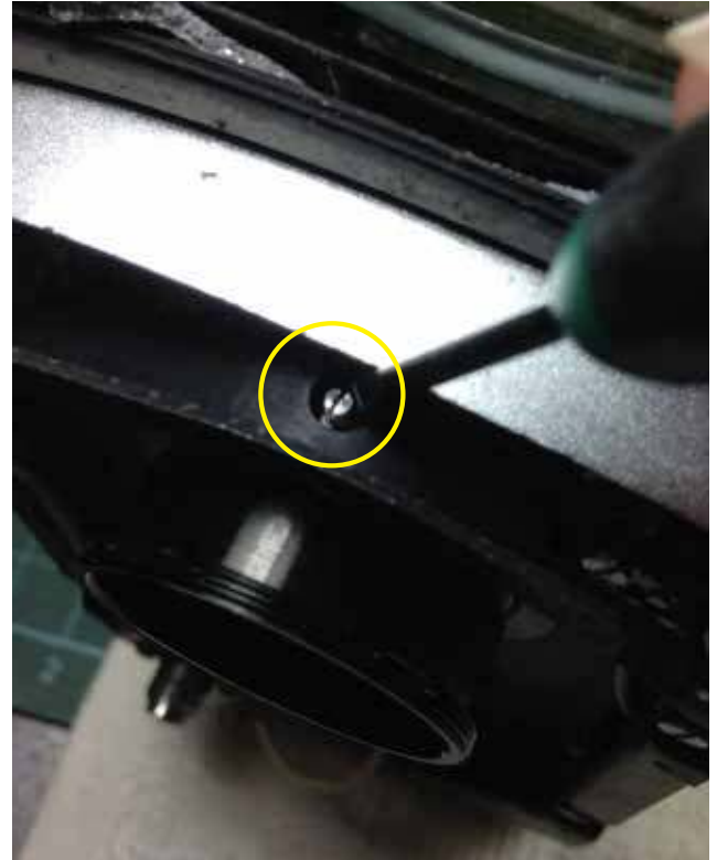
04: I realised during the process that you can skip removing the viewing lens prior to removing the front plate. See the screw (HL in yellow). That is the focusing stop screw for the viewing lens group. REMEMBER this, as this is part of the focusing procedure during assembly. Otherwise leave it as is and don't touch it.
