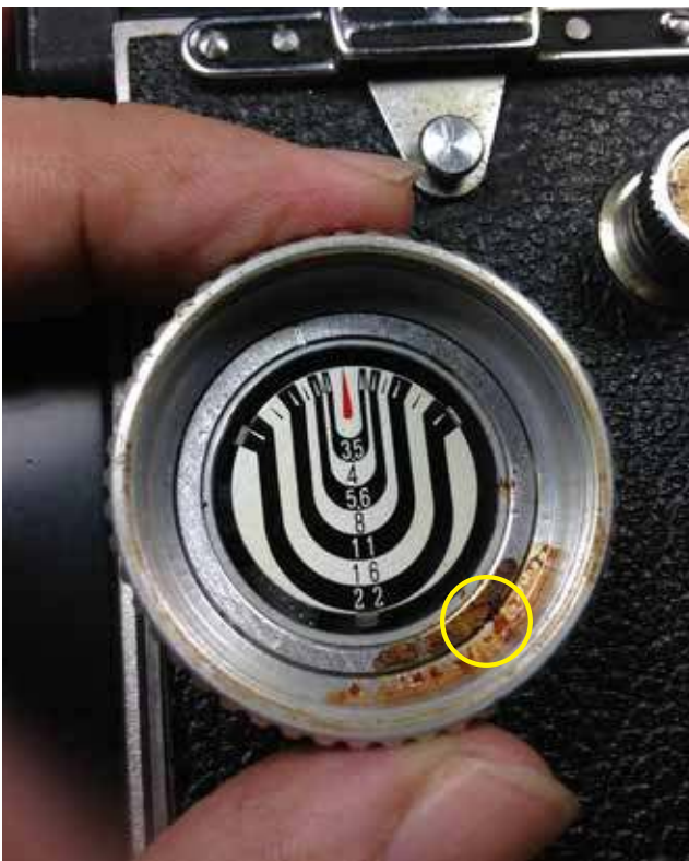
03: Take out the next plastic spacer and you will see this glue residue underneath. I used cotton bud dipped in acetone to wipe it off. Avoid touching the printed scales.
