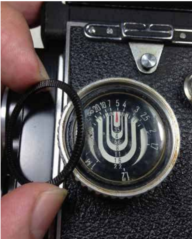
01: Start with removal of this plastic retaining ring. Use a good rubber grip if not use the flatside of your lens spanner. Be careful as you might slip and dent the plastic grooves.
