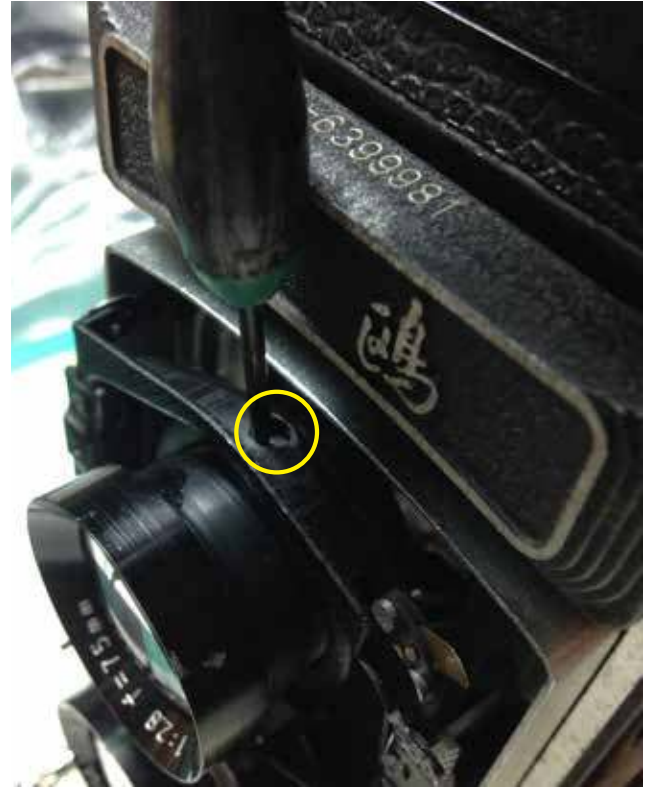
17: Moving on to the viewing lens, there is a stop screw HL in yellow above the lens assembly. Loosen it without removing it, just enough so the lens can be rotated either left or right.
