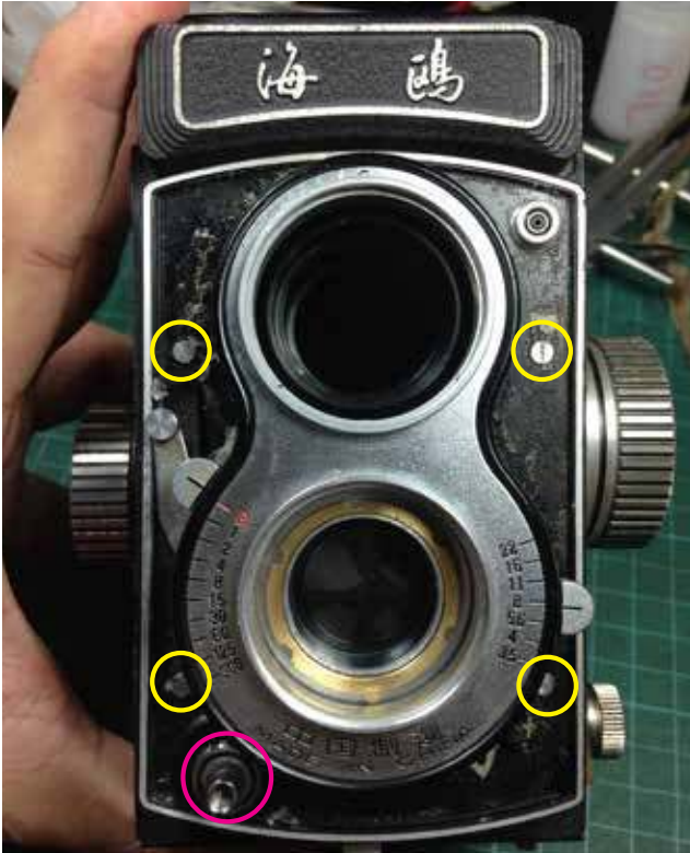
07: Once lenses and leather are out study the front plate. There are four flathead screws on each sides (HL in yellow) remove them. It pays to note which screws belongs to which sides. Unscrew the shutter button retaining ring (HL in red) on lower left using lens spanner or pinhead pliers.
