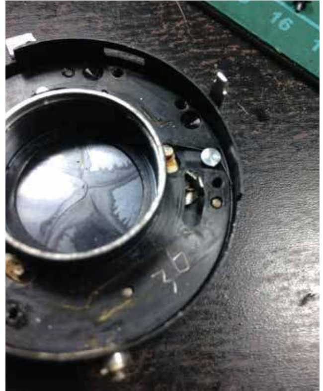
02: Once removed you can wiggle the whole upper part and take note how it goes back. Clean it and set aside.
