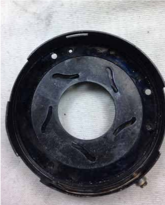
09: Before the re-assembly make sure this two metal parts are also cleaned and dry. Blow dry them if necessary. And once you're confident that all are nice and cleaned you can proceed with the re-assembly of the aperture blades.
