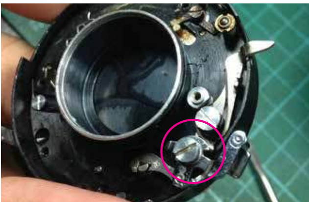
15: Once the first lever is out HL in yellow proceed with the cocking lever HL in red. This is where a big problem appears on this unit.
