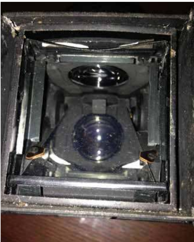
03: If your mirror is like this then you're in luck. It only needs light cleaning. Start with air blower on all corners. I do this upside down so dust will fall off. Then follow it up with light brushing (use soft brush). If in case there are stubborn dirt on mirror use cotton bud dip in lens cleaner or alcohol. Never touch the front mirror surface with your bare fingers. If you can use latex gloves.
