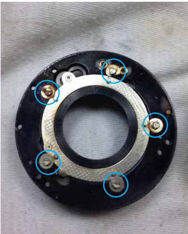
03: Take out this plate. This is the assembly that open and closes the shutter blades. Take note of those HL in blue that holds it down to the metal plate. At this point before removing, try to see how the pivot points rotate. The Stainless Steel (SS) ring rotates as you move the pin on both sides.
