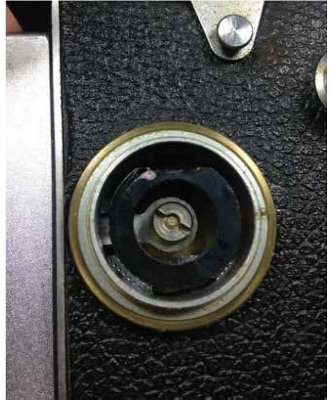
09: While doing this you can then remove the big knob and reposition it later for for the appropriate scale.
