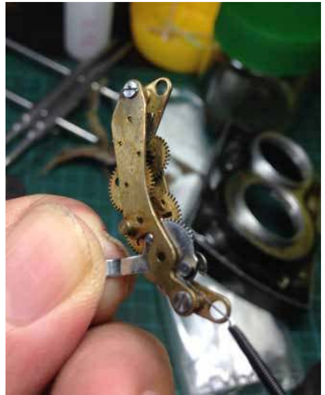
06: Inspect the ST escapement mechanism. Make sure it works. This one has some rust spots and needs light scraping. Do note where the spring was placed. You might need to de-rust this parts using whatever available means you can. I have a dremel so it helps.
