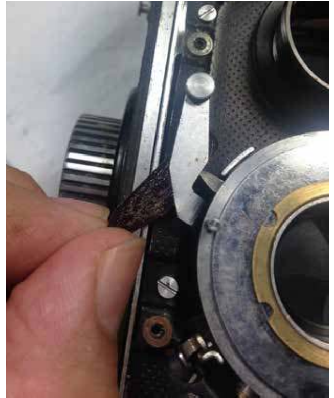
10: Do note there is a hard plastic part just below the cocking lever. It is necessary to place it back once you glue back the leather.
