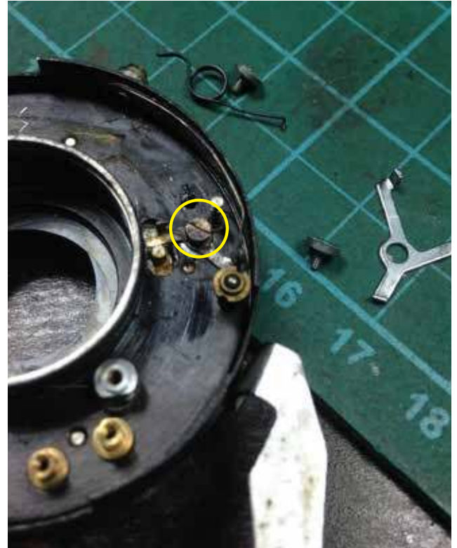
20: Afterwards work on this actuating lever HL in yellow. This activates the shutter blades once released. It's rusty so might need to scrape using wire brush.
