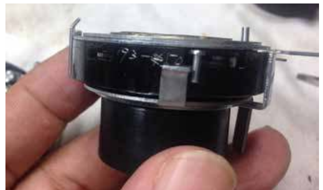
08: After removal of shutter inspect the position of the levers from the back side. For both the aperture and speed levers.
