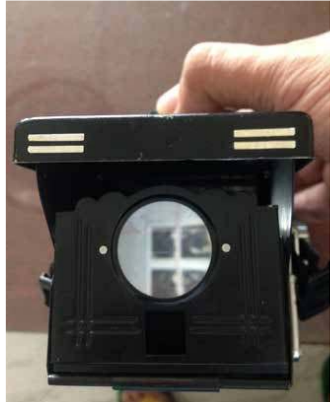
19: Use the magnifier to view it up close and make sure the infinity is sharp and double check the taking lens as well if the infinity is in focus. If both are correct try to view it in close focus too. Usually it is right but if necessary you might need to compensate a bit to have the best focus spots for both infinity and close focus. Afterwards, tighten everything and put all back in reversed order. Congrats!
