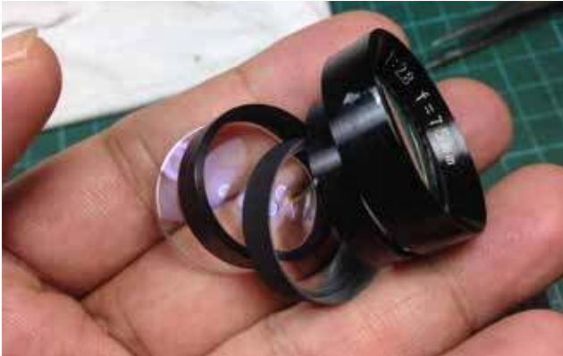
01: Remove the front (viewing/taking) lens elements. I used a furniture rubber feet that matches the retaining ring size of each lenses. When it's not budging put drop of alcohol all around the edges of the ring and wait a few minutes. Make sure to wipe of excess so not to damage markings. Set aside lenses.
