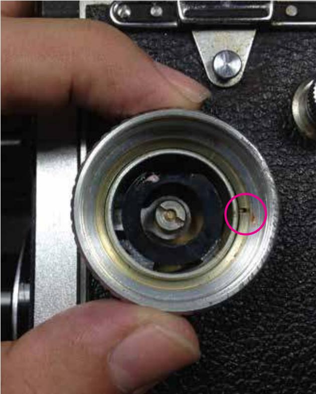
08: Rotate the knob left or right to see how it goes. This make the focus rail move up and down. Do this and do step #15 afterwards. Each time you adjust accordingly to set focus properly.
