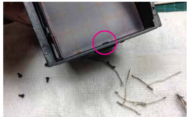
08: Once mirror is out you need to clean them. I did wash it first using water & dishwashing liquid soap. I dried and did one more lens cleaning wipe for good measure. If all cleaned, its time to put them all back in reverse order.
