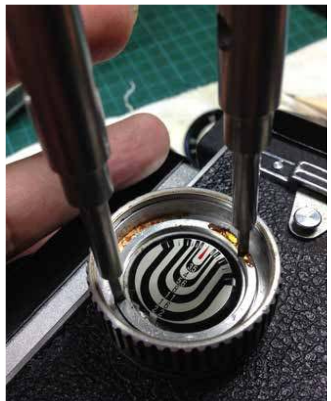
04: Use a lens spanner counterclockwise to remove the ring for the scale. Afterwards you will see there is some sort of metal bent clip (x3) around the scale. No need to straighten them, scale can be taken out easily.
