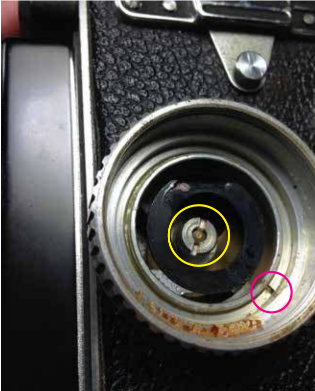
06: This where you need a bit of ingenuity, the middle part with a slotted center HL in yellow, you need to loosen. Take note of the position of the slot in the knob HL in red. This is your guide for the infinity mark.
