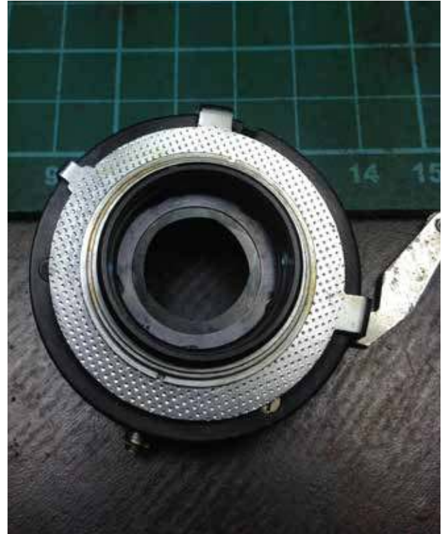
24: Now this is where we separate the men from the boys. If you want to proceed working on the shutter and aperture blades you can carry on Part 2b. Otherwise just proceed to clean the blades on both side of the shutter with lighter fluid while flushing the dirts and grimes. I used brush and blower. This might be tricky as you'll never know whats the condition of the internal parts?
