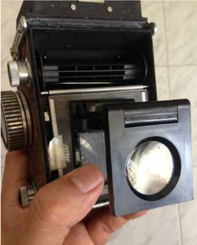
14: Use a magnifying loupe or similar to view the ground glass. What you need to set on the shutter is put it on B setting, the widest opening (f3.5) and trip the shutter and hold it either by putting cell tape or using shutter release with lock.
