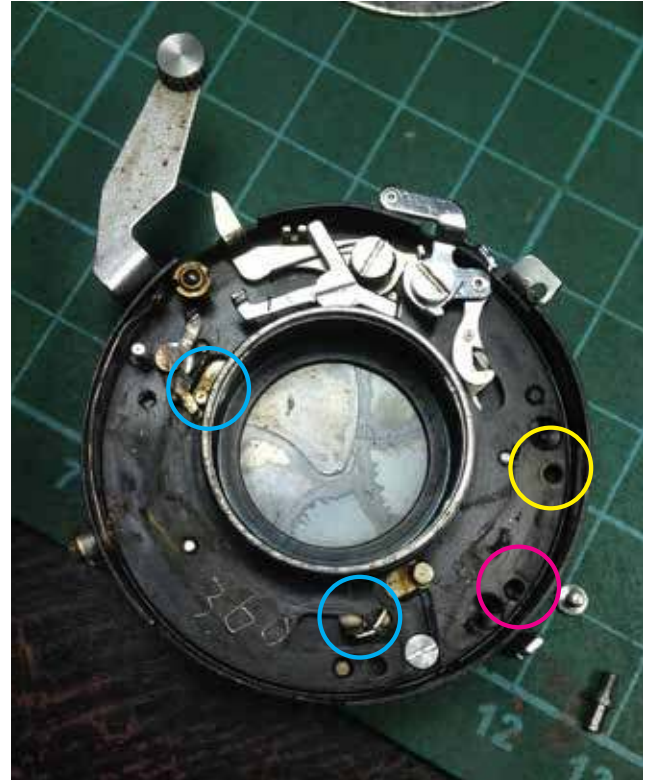
12: Now the big mechanism is gone you can see the smaller lever and pivoting parts on top. I HL the position here of the mechanism. This is where you can test of the blades by moving the lever points HL in blue. If yes, it is a good sign and it just needs cleaning up. Mine is stucked up so I must proceed further than this stage here.
