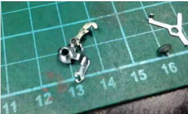
17: Now to carry on with the build, assuming we have the spring for the cocking lever. See different views of the lever.
