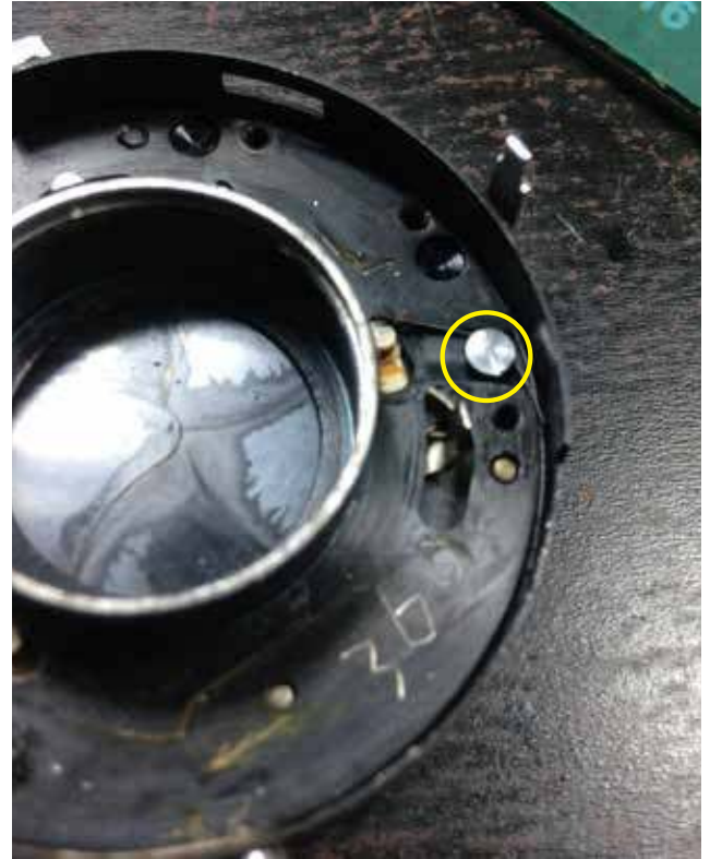
22: At this stage all of the upper parts of the shutter are removed except this one HL in yellow. This is the return spring once the shutter is activated. It makes the blades return to its closed position.
