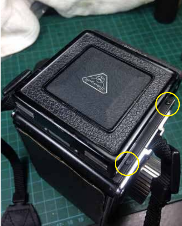
01: Start by removing 4 screws HL in yellow, 2 on each side. As always try to note how the parts work and where it goes prior to removal.
