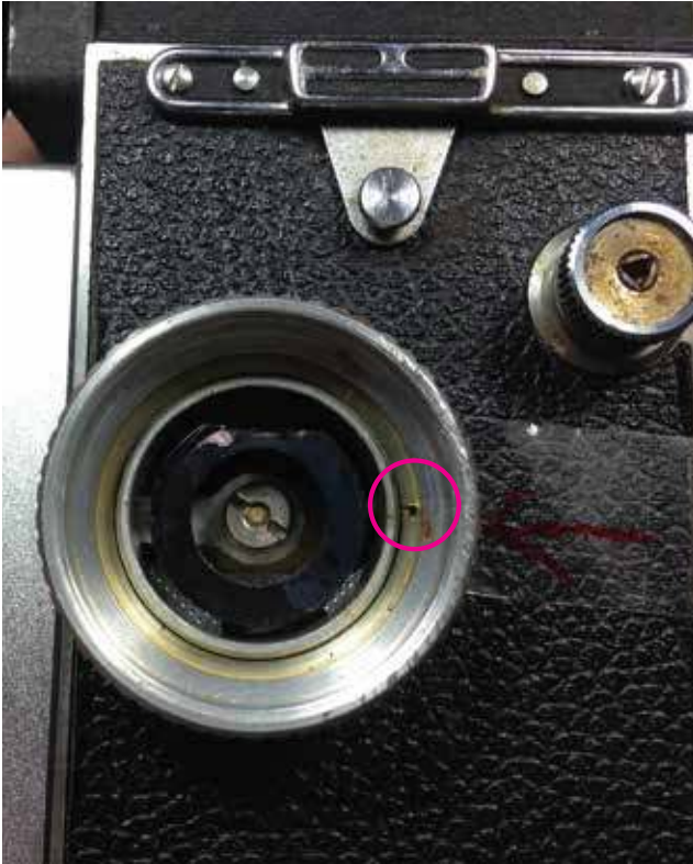
16: Once you hit the perfect focus mark the slot as mentioned HL in red and now it is set to infinity. You can now tightened back the slotted screw and make sure it is secured without moving the knob.
