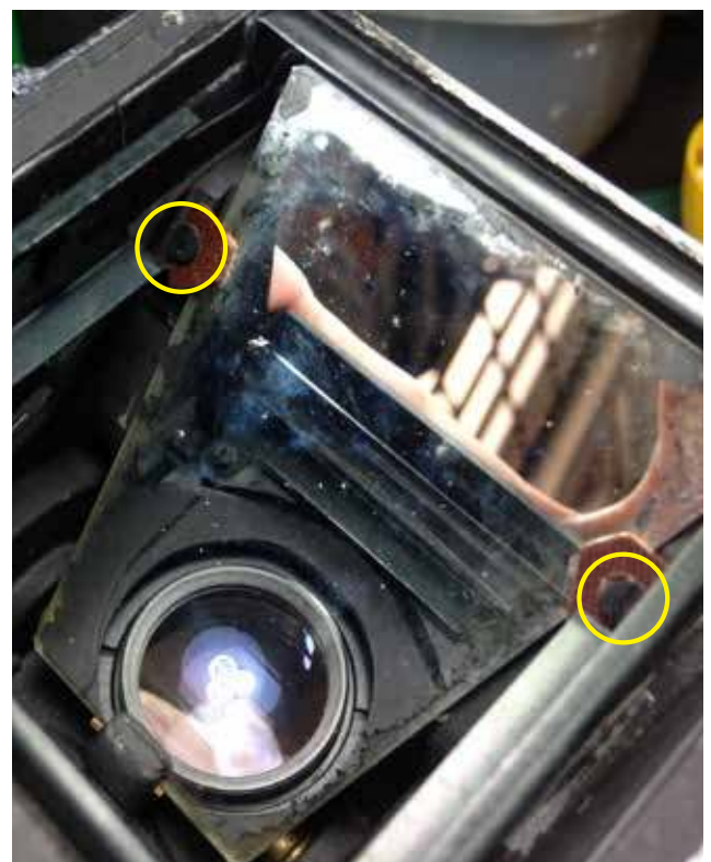
04: Do it gently as this is a front surface mirror and the reflective part can be easily scratched. Test on edges first before going through other portions. There is really not much you can do here if you cant remove the stains. Replacement mirror is your options. In which case all you need to do is remove two screws on the side HL in yellow and replace the mirror.
