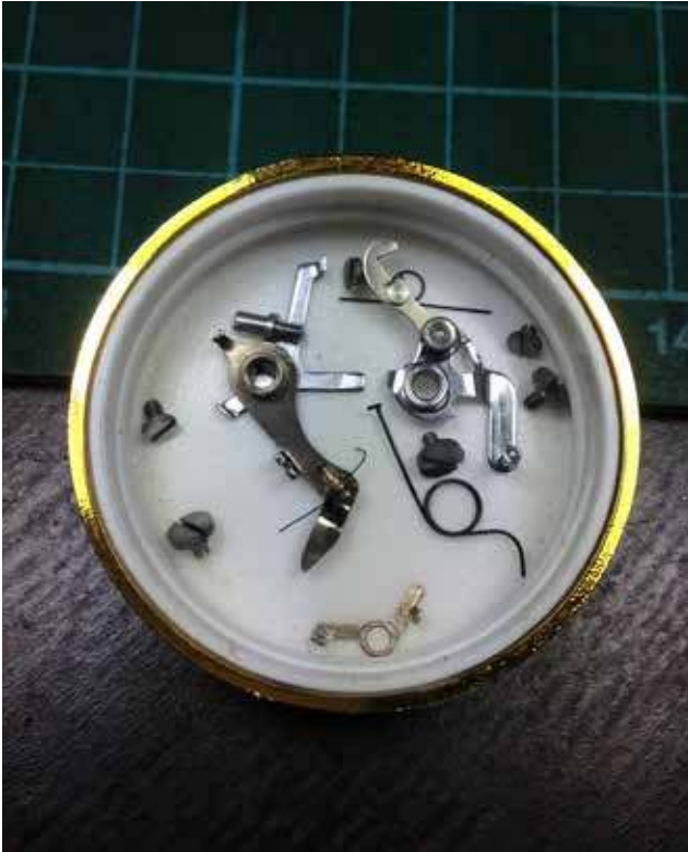
23: I placed all the parts in a bottle cap after I cleaned them one by one. I make it a practice to clean them immediately after they are removed. This is a good time to check for some bent or mis-aligned levers.
