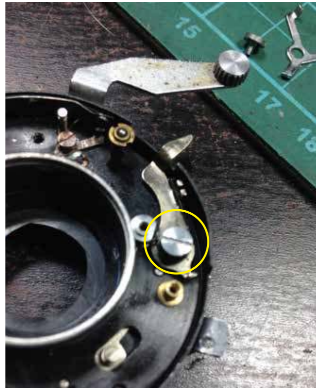
18: Next to be removed is the shutter release lever. Loosen the screw HL in yellow.
