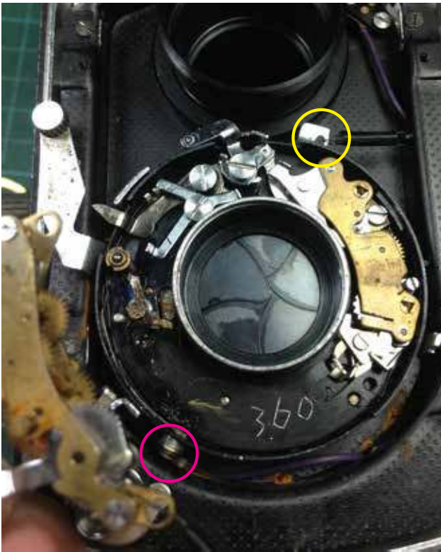
05: Remove the ST mechanism. See the HL in red remove the flash sync post. Be careful as the screw is tiny. Once cable is out placed the screw back. The HL in yellow on top is the spring that holds back in position the cocking lever, detached them and make sure it wont fly out.
