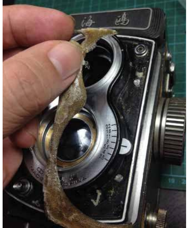
06: Remove leather on each side carefully. Sometimes you might need to use alcohol to loosen the glue. But in this case I inserted a thin artist spatula and work my way underneath to remove the leather. NOTE: some camera has brittle leather so remove at own risk. Store the leather inside book pages to flatten while working on the camera.
