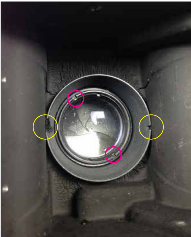
07: At this stage I decided to detached the whole shutter assembly from the body. Start by removing the back lens group using lens spanner HL in red. Afterwards you can remove the retaining ring HL in yellow. Do note that at horizontal position the notch is touching the interior sides. Be careful turning it counterclockwise while holding the lens spanner as this might slip.
