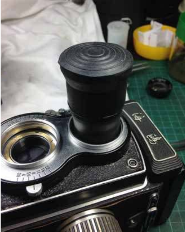
01: Remove the front (viewing/taking) lens elements. I used a furniture rubber feet that matches the retaining ring size of each lenses. When it's not budging put drop of alcohol all around the edges of the ring and wait a few minutes. Make sure to wipe of excess so not to damage markings. Set aside lenses.
