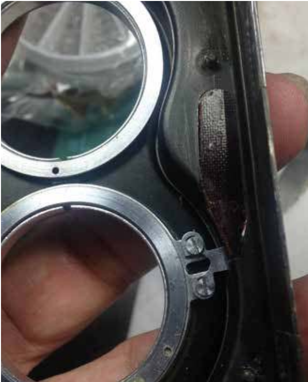
11: The interior side where you can see the plastic part covering the cocking lever side.
