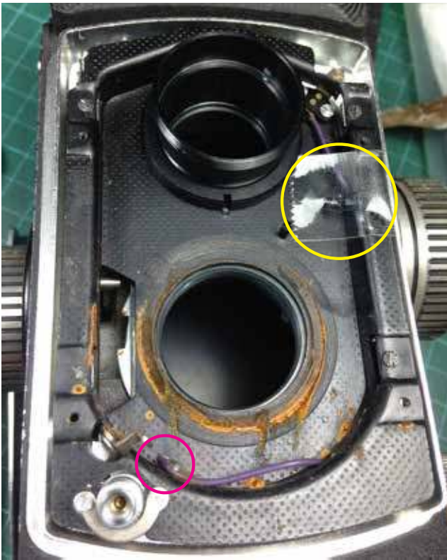
09: The front base plate of the focus rails now is shown. With rusts all around. Time to use my dremel to good use and then touch up with paint. Note the loose spring HL in yellow I used cell tape to keep it. And the sync cable HL in red.
