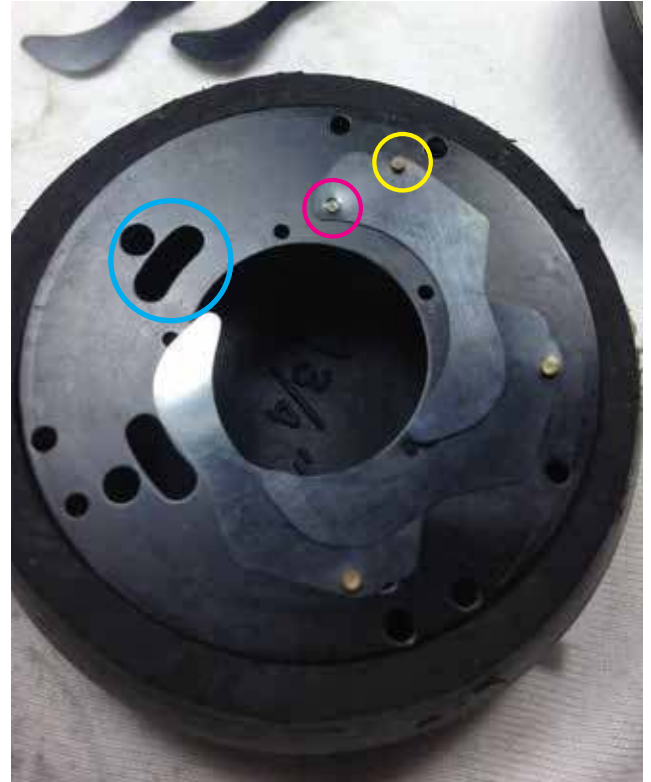
10: Now do the re-assembly of the blades take note of those pivots points HL in yellow & red. And the HL in blue where the pivot RED goes. I used a furniture rubber as a base to elevate the plate. Start with one point and do them one after the other. I did it counterclockwise. There are five blades and the first 3 should be easy.
