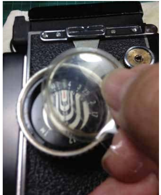
02: Take out the plastic dome. If it doesn't fall off by itself use a cell tape to grab it.
