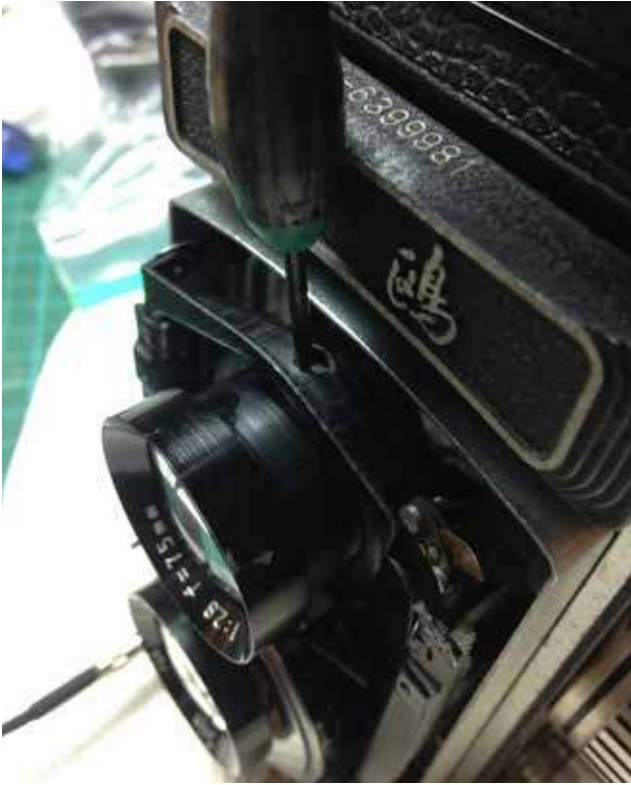
05: If you decide to do this part then loosen but don't remove the screw. Just enough so you can rotate the lens unit counterclockwise.
