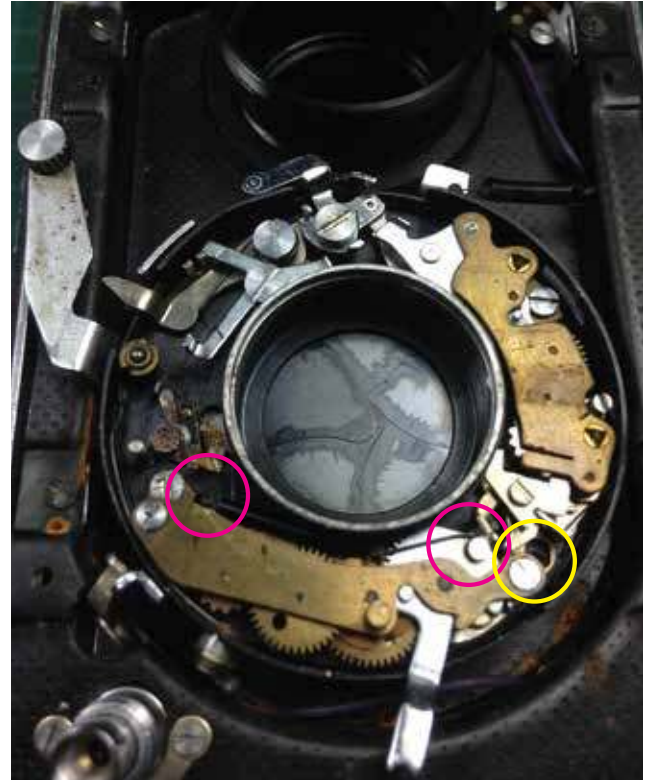
04: I noticed one missing screw (HL in yellow) for the ST mechanism. The one HL in red is the spring that holds back the ST lever to its starting position. You can detached it for removal. After inspection the ST on this one works but the Slow Speed Escapement (SSE) on right does not.
