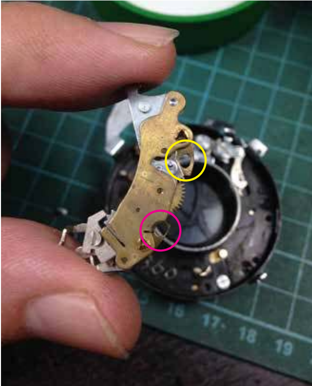
11: Now proceed to remove the SSE mechanism by removing two screws. Note that one screw is longer than the other HL in red. Take note of the position where it goes back. It is important as minute increment to left and right affects the speed. What I did is to mark the base metal and inscribed with pointed tool.
