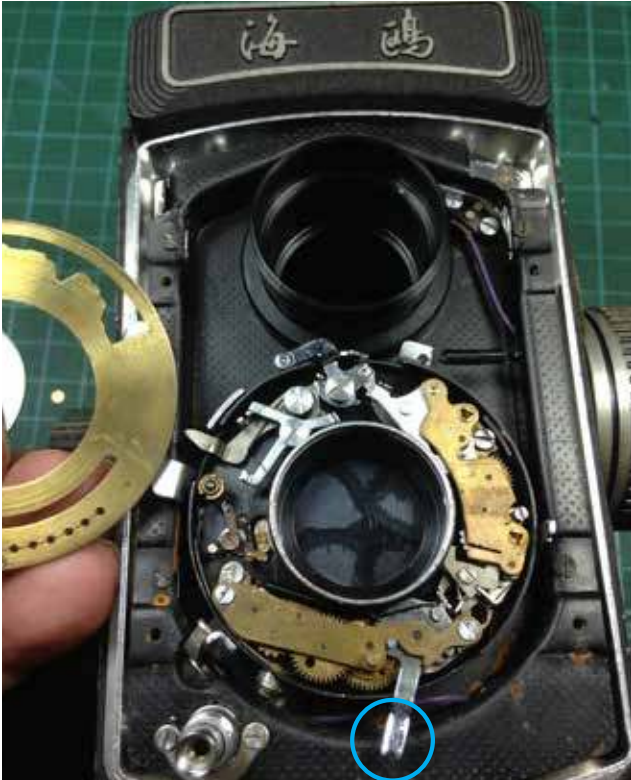
03: Remove the speed plate and then you can now see the internal parts of the shutter mechanism. Study them and do a visual inspection of the parts. Overall oily, dirty and some rust here and there. HL in blue is the missing knob for the Self Timer (ST) lever.
