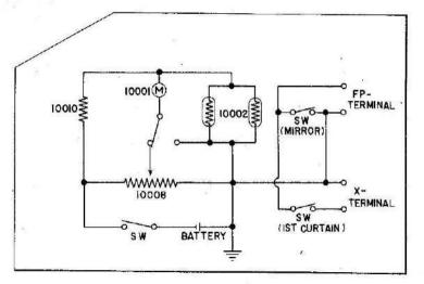
Exposure meter circuits for Asahi/Honeywell Pentax SP (Spotmatic), SP-F (Spotmatic F) and KM. The circuit diagrams are from Asahi Optical Co. service manuals.
