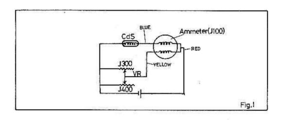
When the current value of CdS side becomes larger than VR Cds何の電流がVR例より大きくなると、 side, the needle of Ammeter (J100) goes up.
