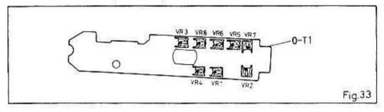
VR1 &. VR4: These two resistors should never be adjusted in servicing
