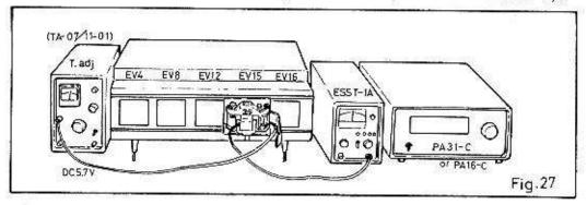
Put the camera on the camera stand equipped with light value correction unit. Set the camera as shown in Fig. 27
