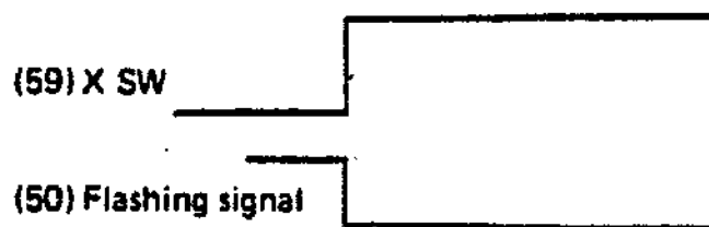
Time chart of X SW ON signal and flashing signal
