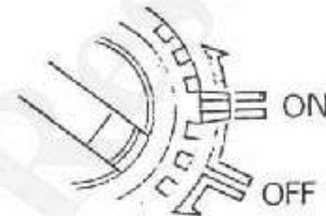
Switch for shutter speed indicating LED unit in viewfinder
