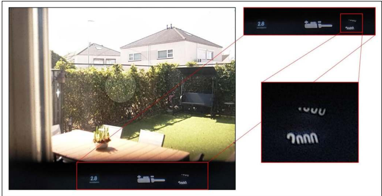
Nikon F2A viewfinder image with on the bottom from left to right: the aperture information, the exposure and the shutter speed information. The two circles show the 60/40 percent center-weighted exposure reading.
