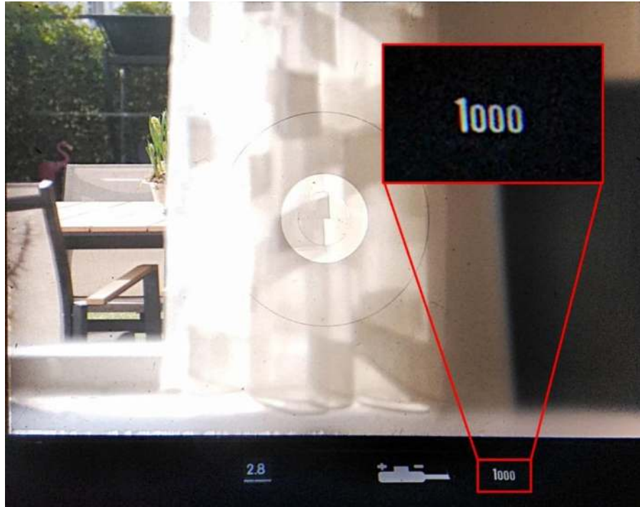
Nikon F2A viewfinder image with on the bottom from left to right: the aperture information, the exposure and the shutter speed information. The shutter speed read out is now aligned.
