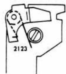
■ Fig. 5 2123 spring setting
