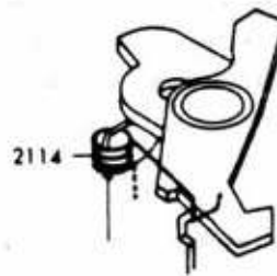
■ Fig. 4 2114 spring setting
