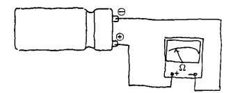
Flashing Test (Checking the trigger circuit)
