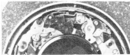
Shutter setting sequence. The topmost picture shows the unset condition. The middle picture shows the set condition. The bottom picture also shows the set condition but with the shutter setting plate back at its original position.
