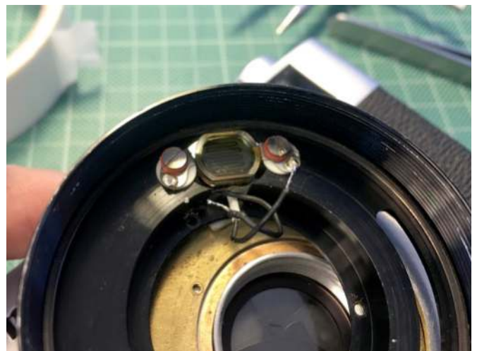
5.3 — Unweld the EE wires
