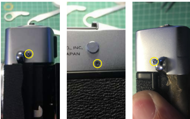
12.2 — Top cover, remove this 3 screws
