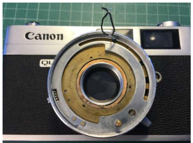
7 — Remove the speeds and ASA/DIN ring
